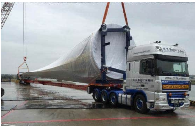
Figure 2-4:Example -Transport of Blades on extendible trailers
