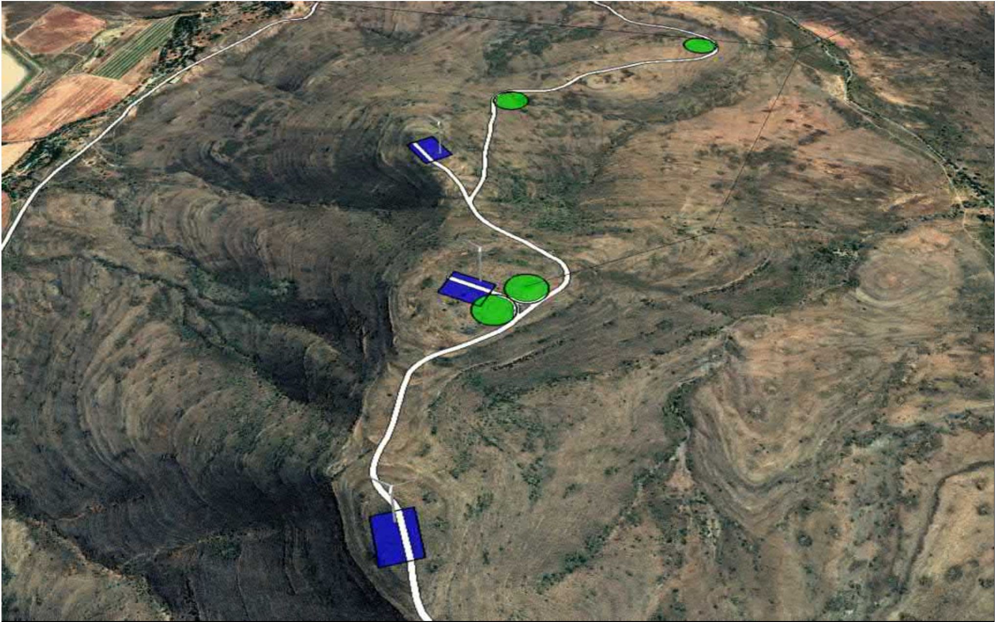
Figure 9 Plateau position of the internal roads/turning circles, laydown areas and turbines at Karreebosch WEF
