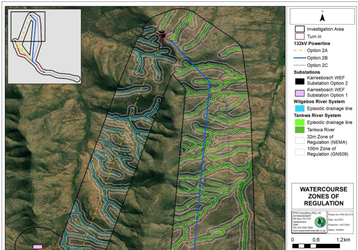
Figure 0-8: The conceptual presentation of the zones of regulation relation to the delineated watercourses that form part of the Tankwa and Wilgebos River system within the northern portion of the investigation area. (Take note due to the scale of the map: Substation Option 2 is located approximately 20m from the delineated extent of an episodic drainage line)
