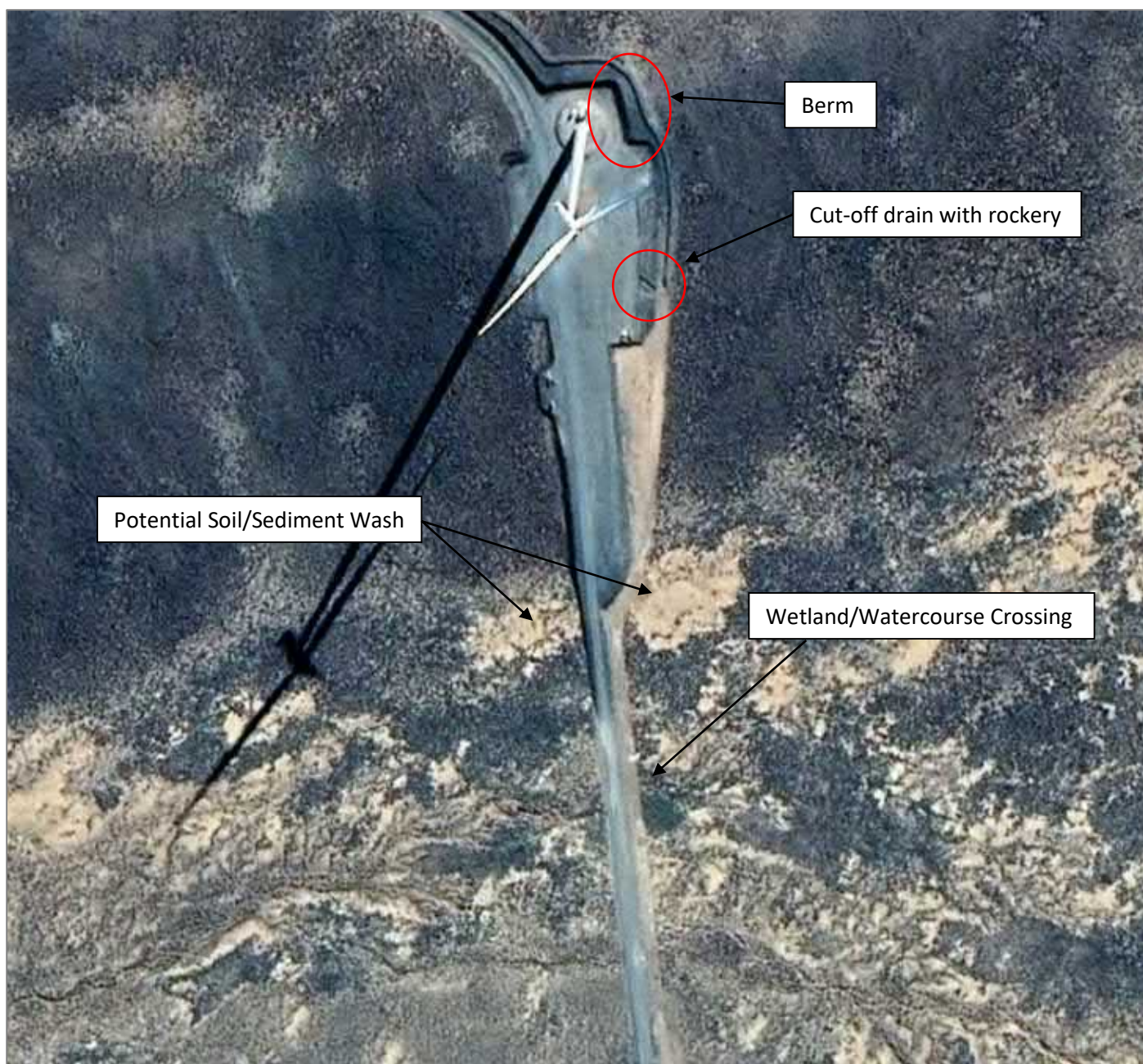
Figure 14 Existing lay-down area and turbine for the nearby Perdekraal site as a comparative example
