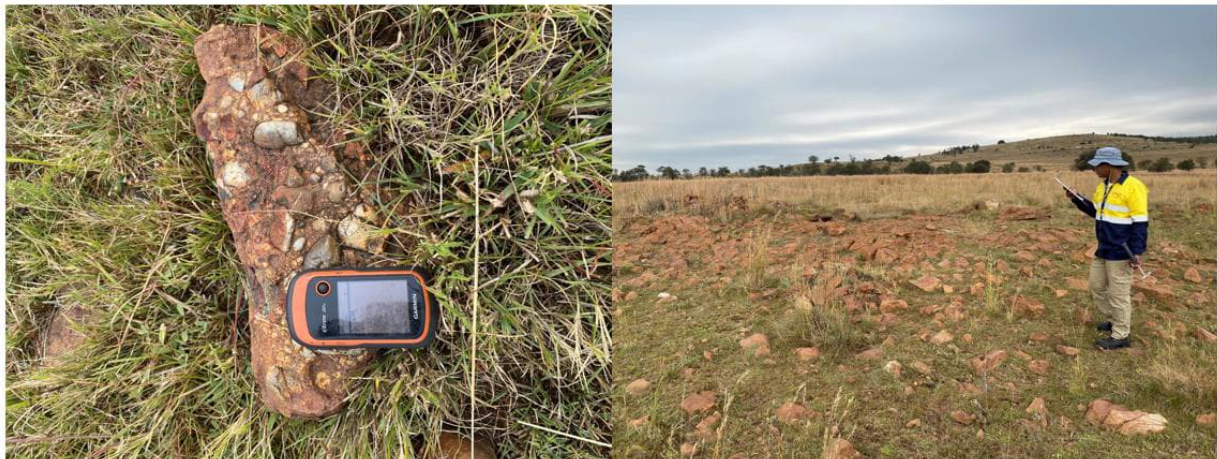
Figure 4-6 - Variability of depth of decomposition in the Hekpoort andesite.
