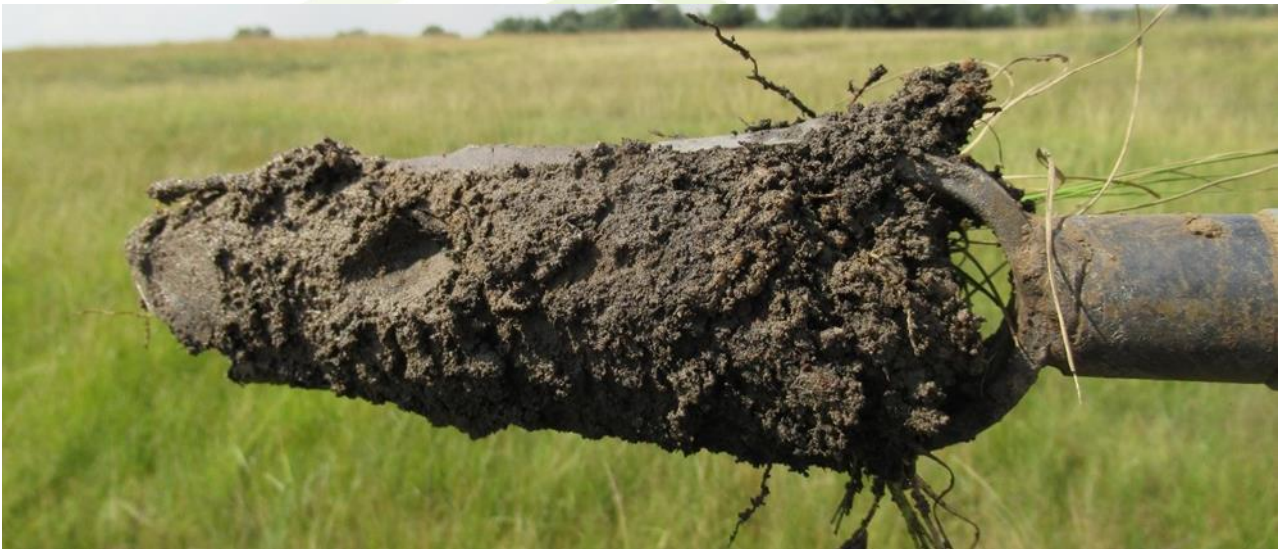
Figure 9.13: Hydric soils included a Sandy Clay Loam soil form associated with the wetland areas
