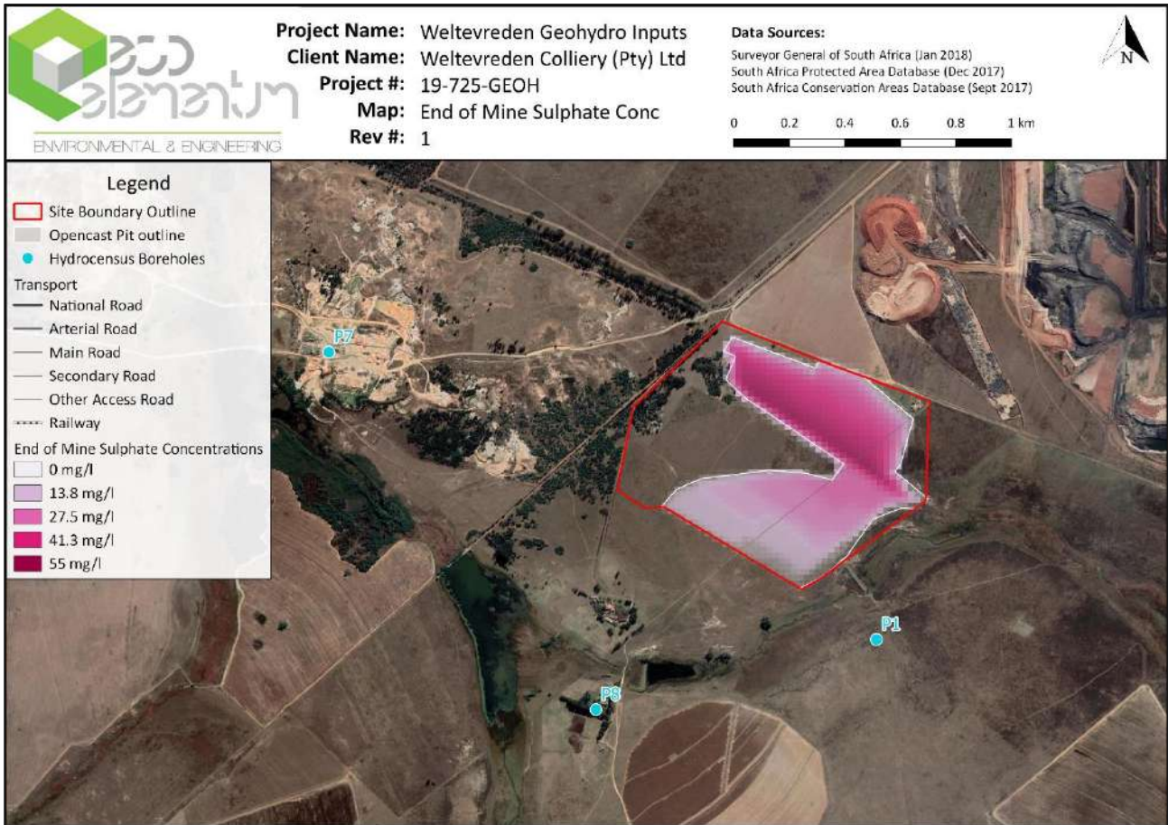
Figure 13.2: The simulated mass transport at the end of the operational phase at Weltevreden Colliery.
