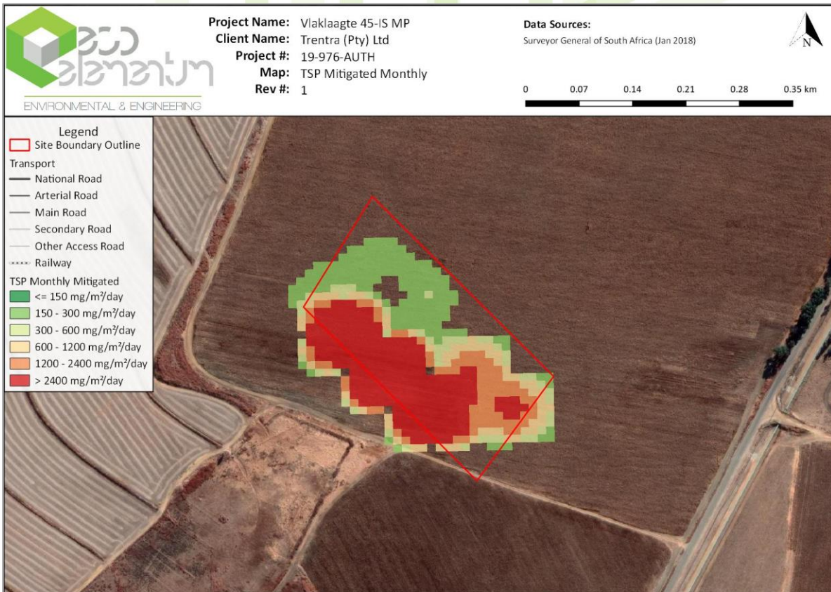
Figure 3.42: Predicted highest monthly deposition for TSP for the proposed Vlaklaagte project operations when mitigated.
