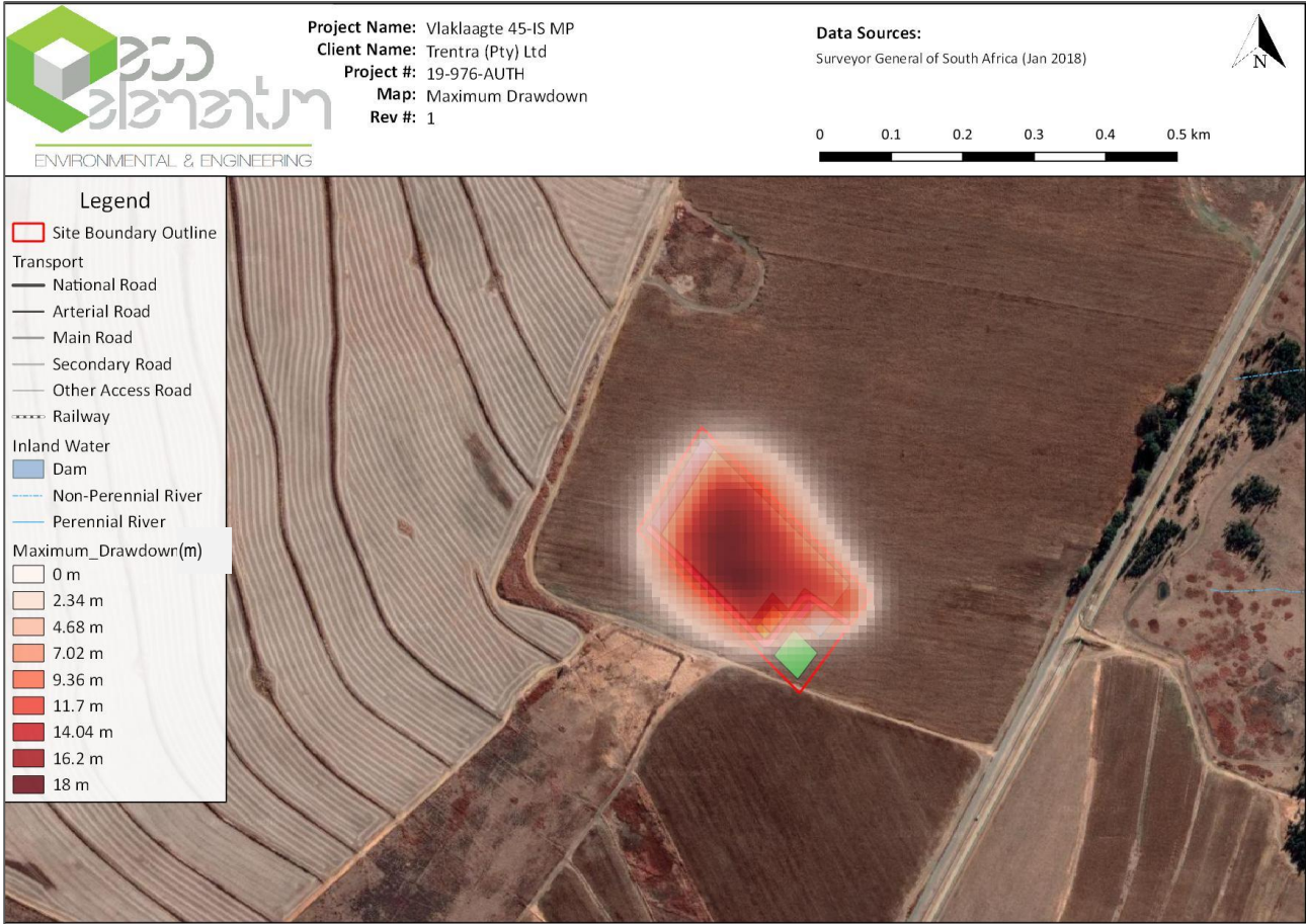
Figure 3.31: Simulated drawdown in the Trentra Vlaklaagte mining pit.
