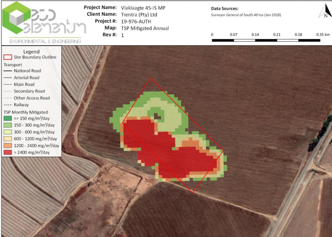
Figure 3.40: Predicted average annual deposition for TSP for the proposed Vlaklaagte project operations when mitigated.
