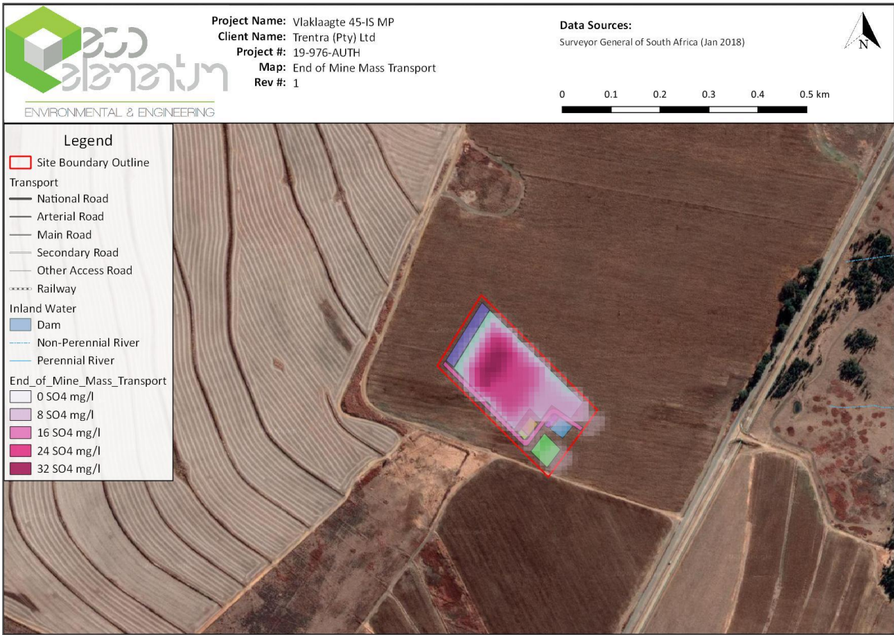
Figure 3.32: The simulated mass transport at the end of the operational phase at the Trentra Vlaklaagte mining area.
