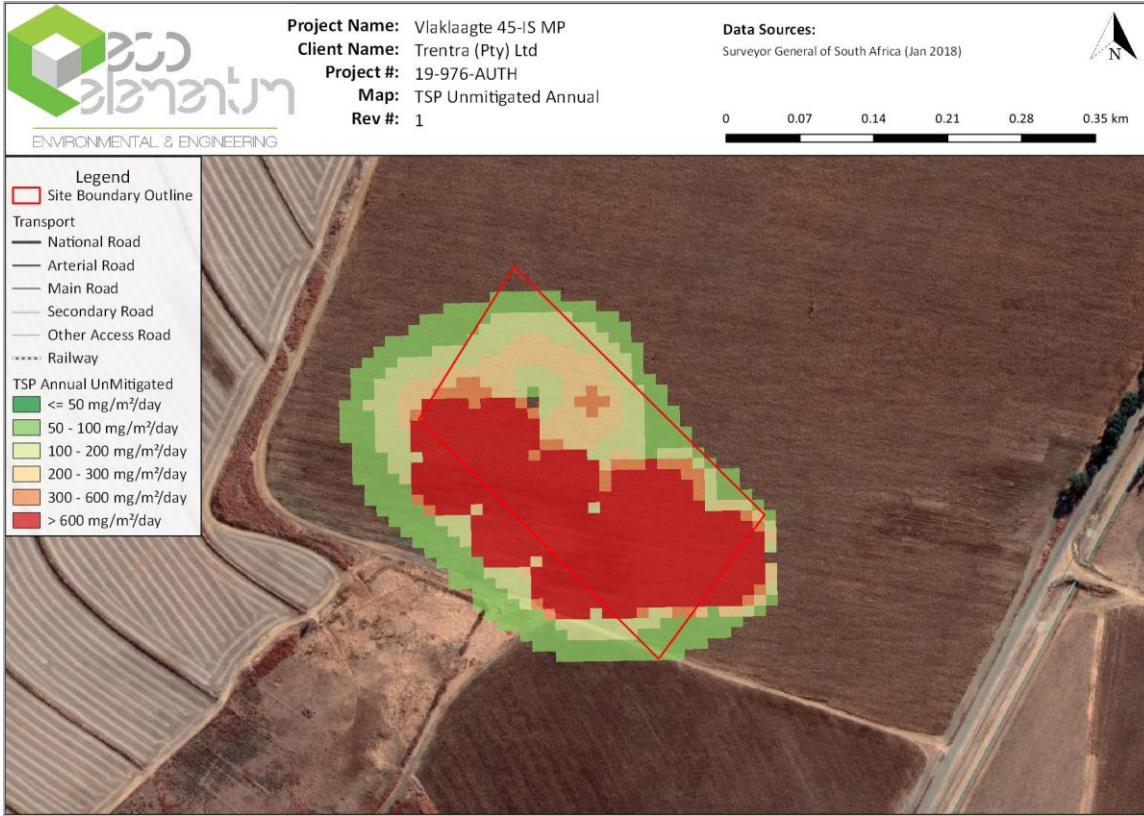
Figure 3.39: Predicted average annual deposition for TSP for the proposed Vlaklaagte project operations when unmitigated.
