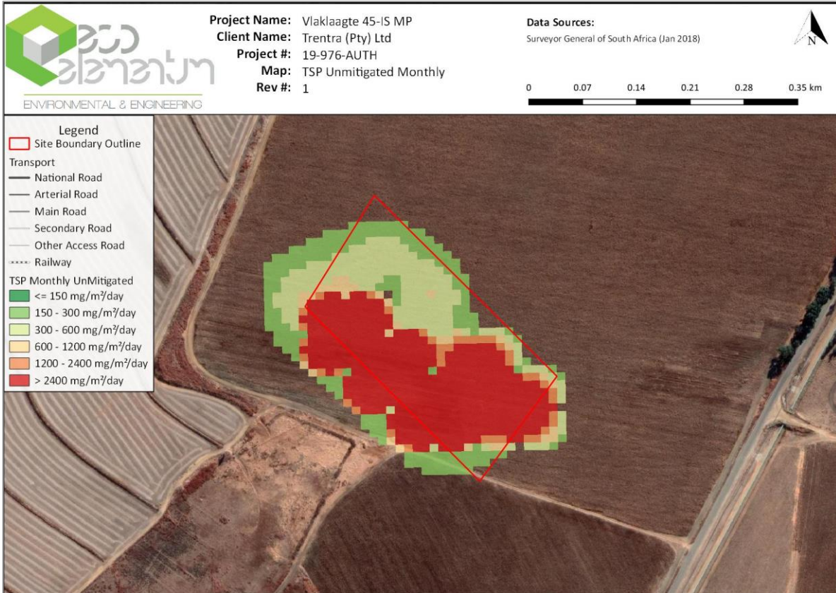
Figure 3.41: Predicted highest monthly deposition for TSP for the proposed Vlaklaagte project operations when unmitigated.
