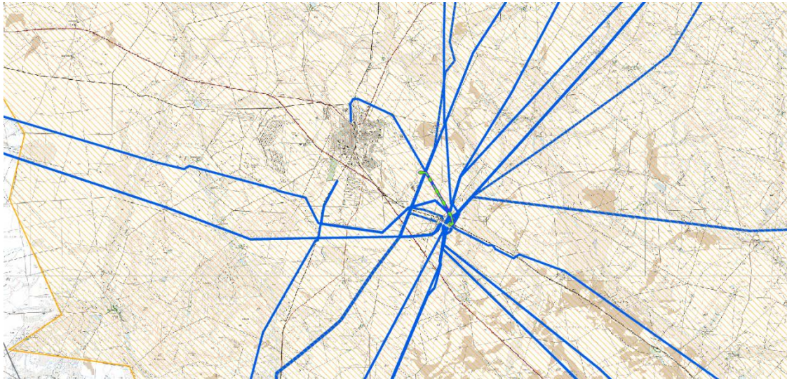
Figure 2: Grid connection corridor (green) in relation to existing electricity transmission infrastructure (blue) converging on the Hydra Main Transmission Substation near De Aar, with a small portion of the large IBA covering a large portion of the region indicated with orange hatching.
