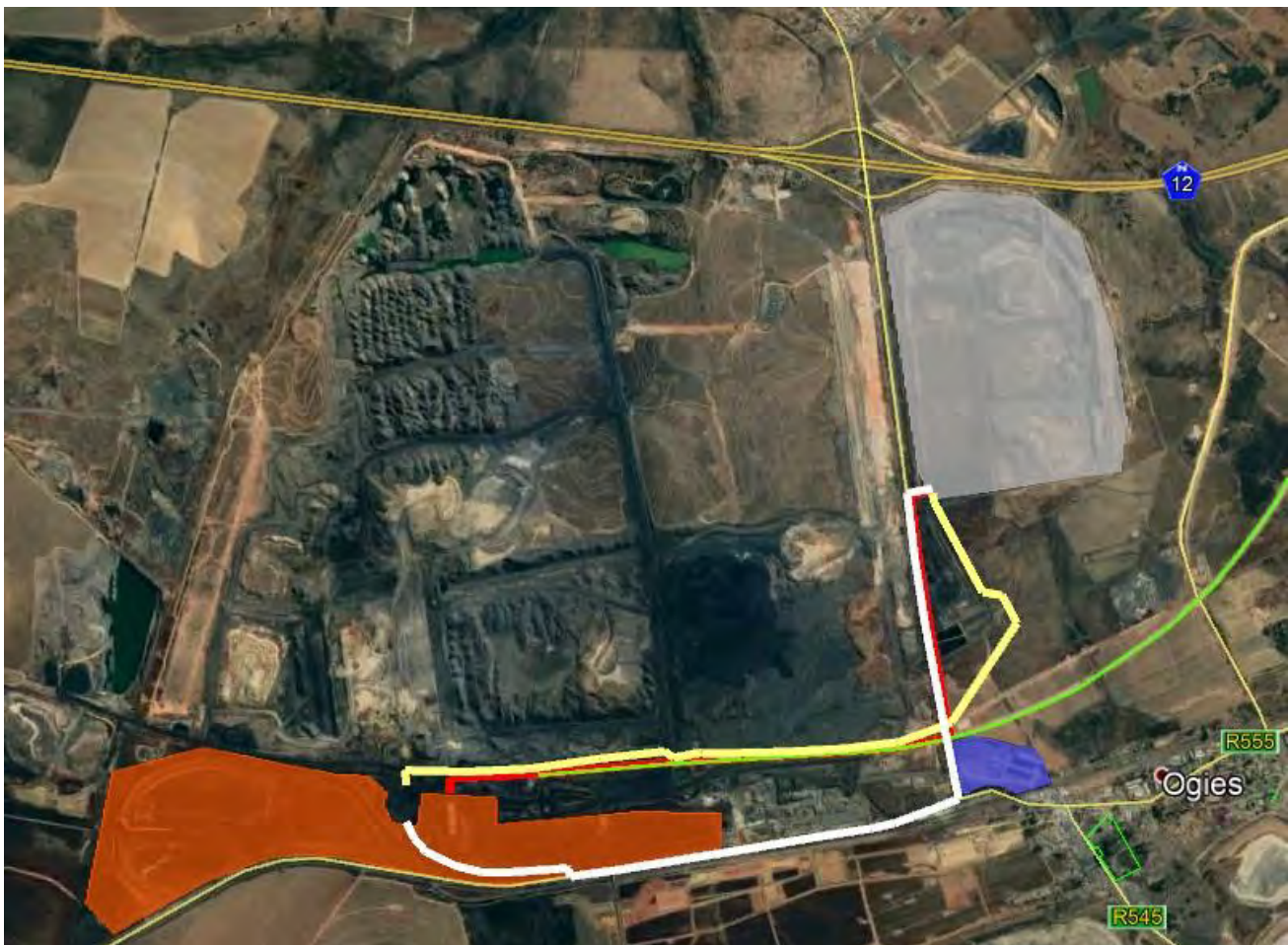
Figure 9: Map indicating conceptual alignment of proposed discard transport alternatives. A public road route in white, a proposed mine road crossing the South32 property in yellow and proposed new conveyor route in red. The alignment of an existing coal conveyor is indicated in green.
