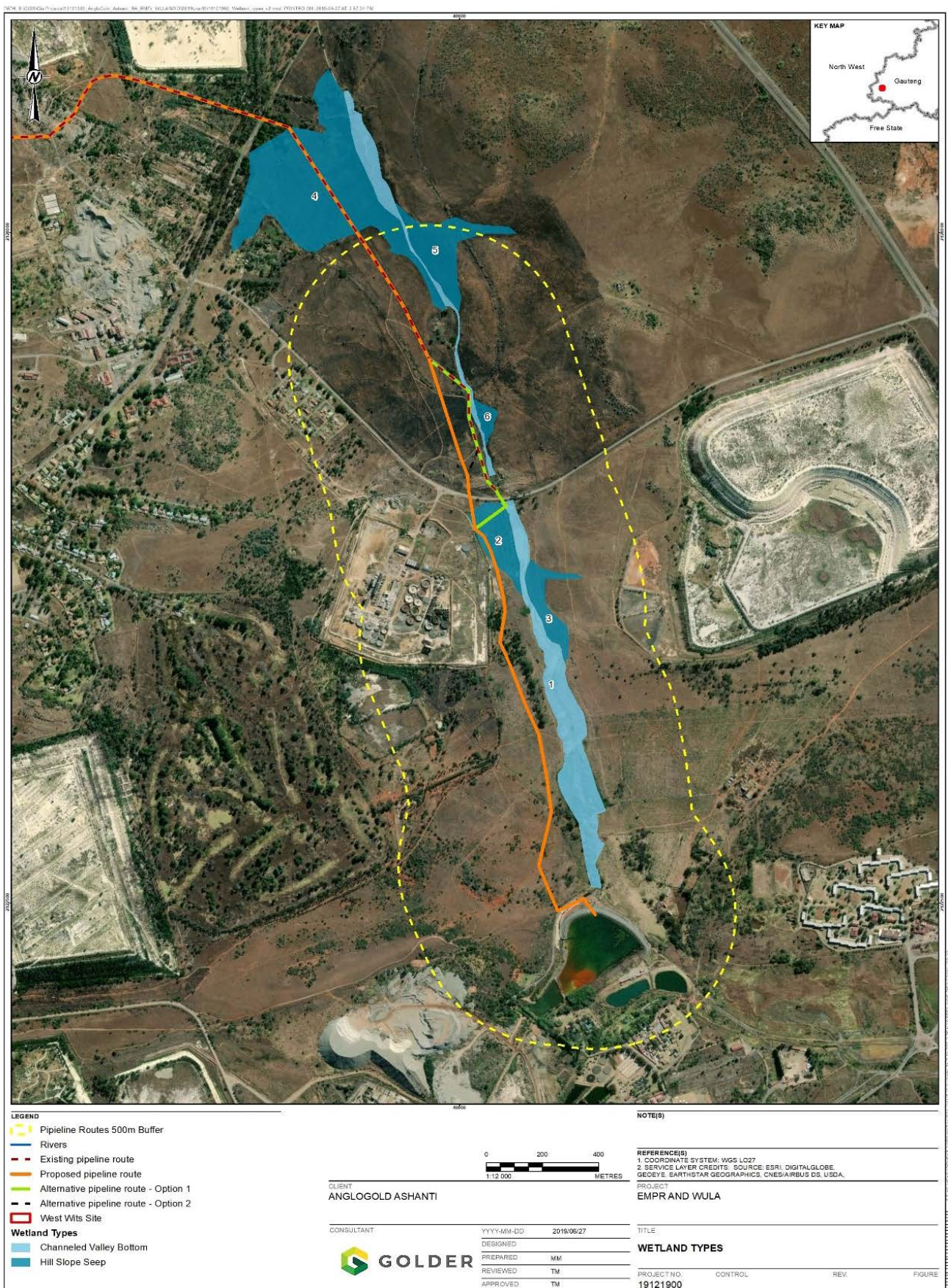
Figure 11: Preliminary desktop delineation of suspected wetlands within 500m of the proposed pipeline
