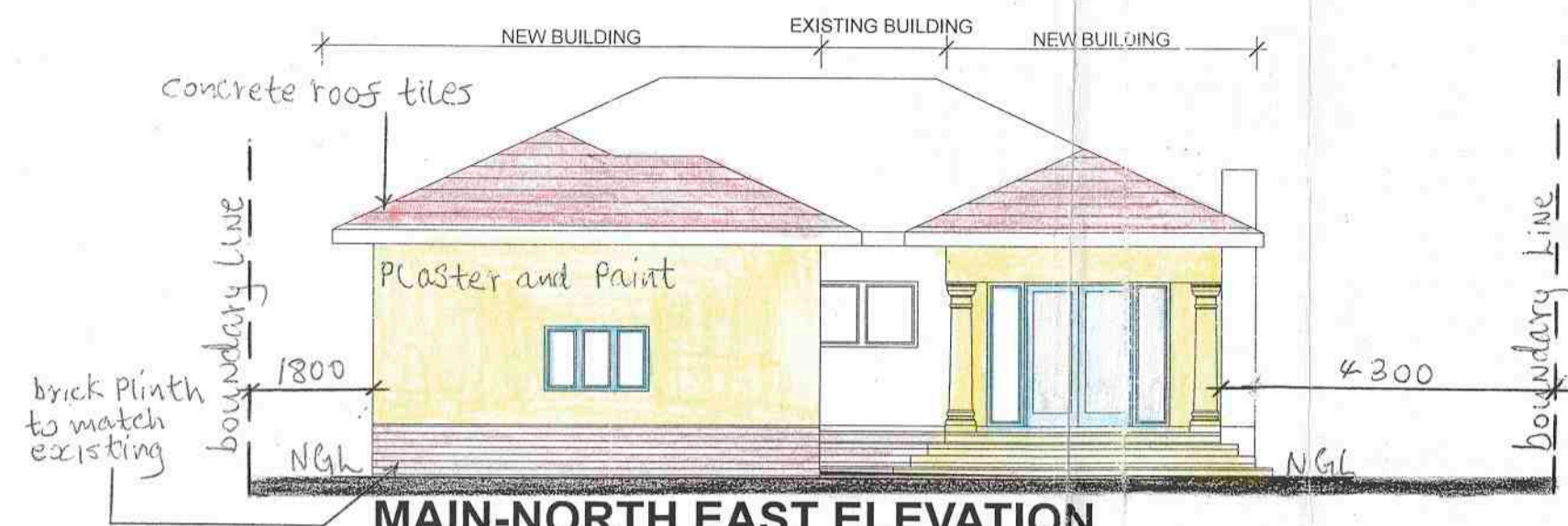
MAIN-NORTH EAST ELEVATION
