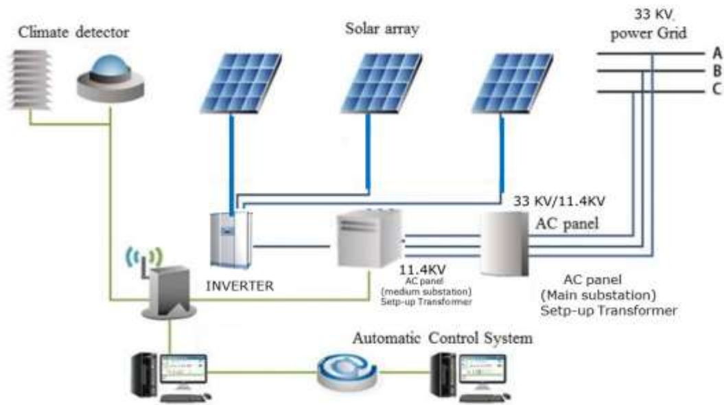
Figure 2: System Design Overview 2
