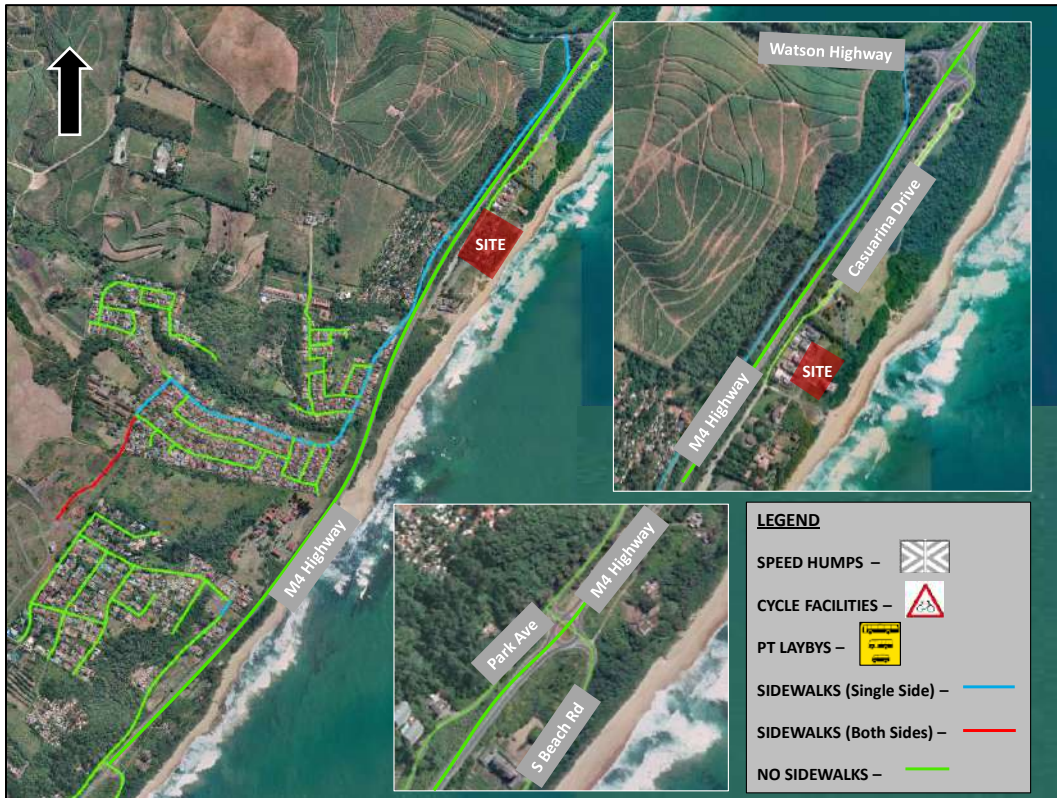
Figure 8: Location of Existing Facilities
