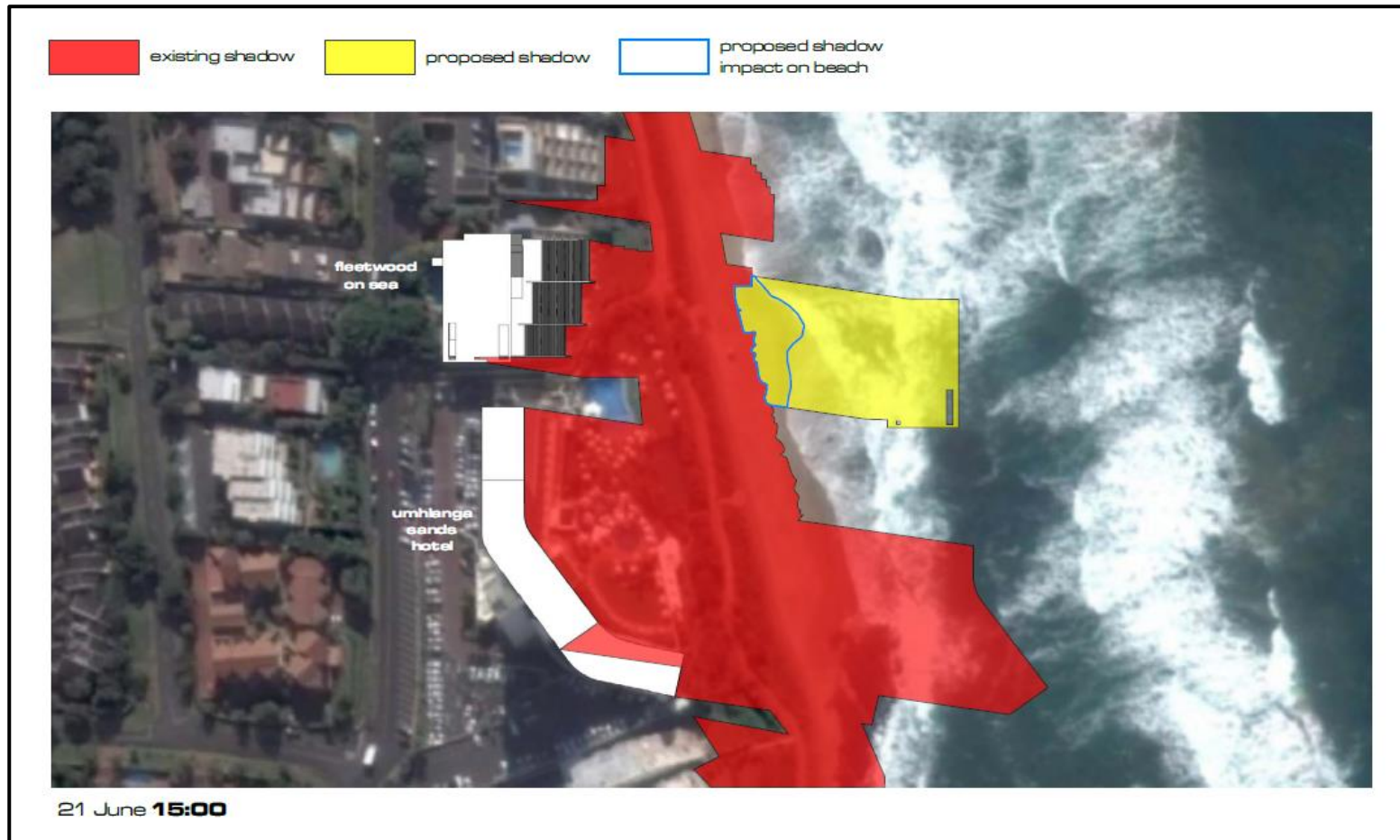
Figure 10: Shadow Impact of proposed building on 21 June at 15:00. The actual additional impact is depicted in blue.
