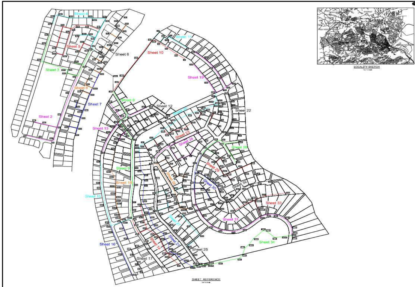
Figure 1: Preferred Layout Alternative for the proposed sewage reticulation
