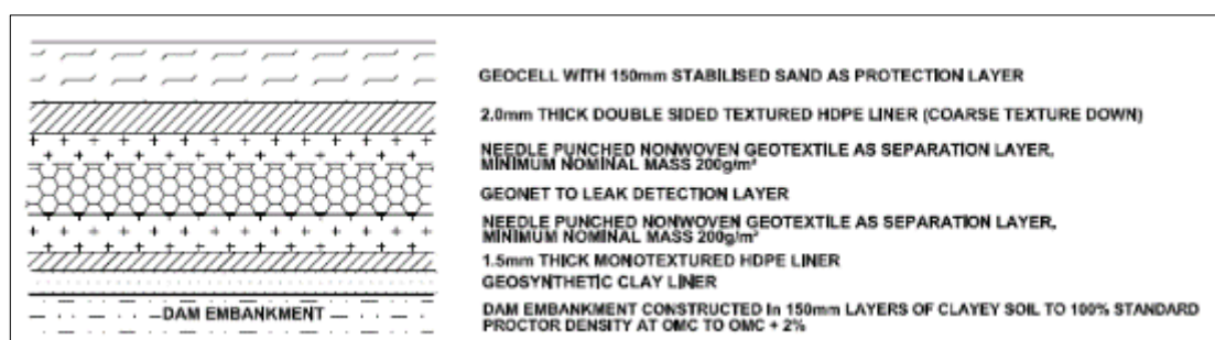
Figure 2-7: PCD Side Slope Liner Detail.
