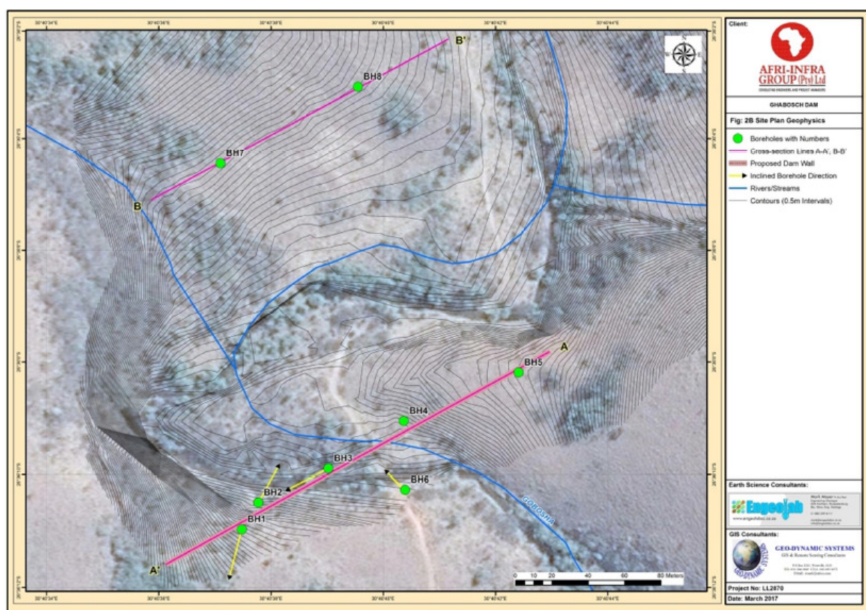
Figure 5.2e: Borehole positions at Dam Site B (taken from Meyer, 2017b)
