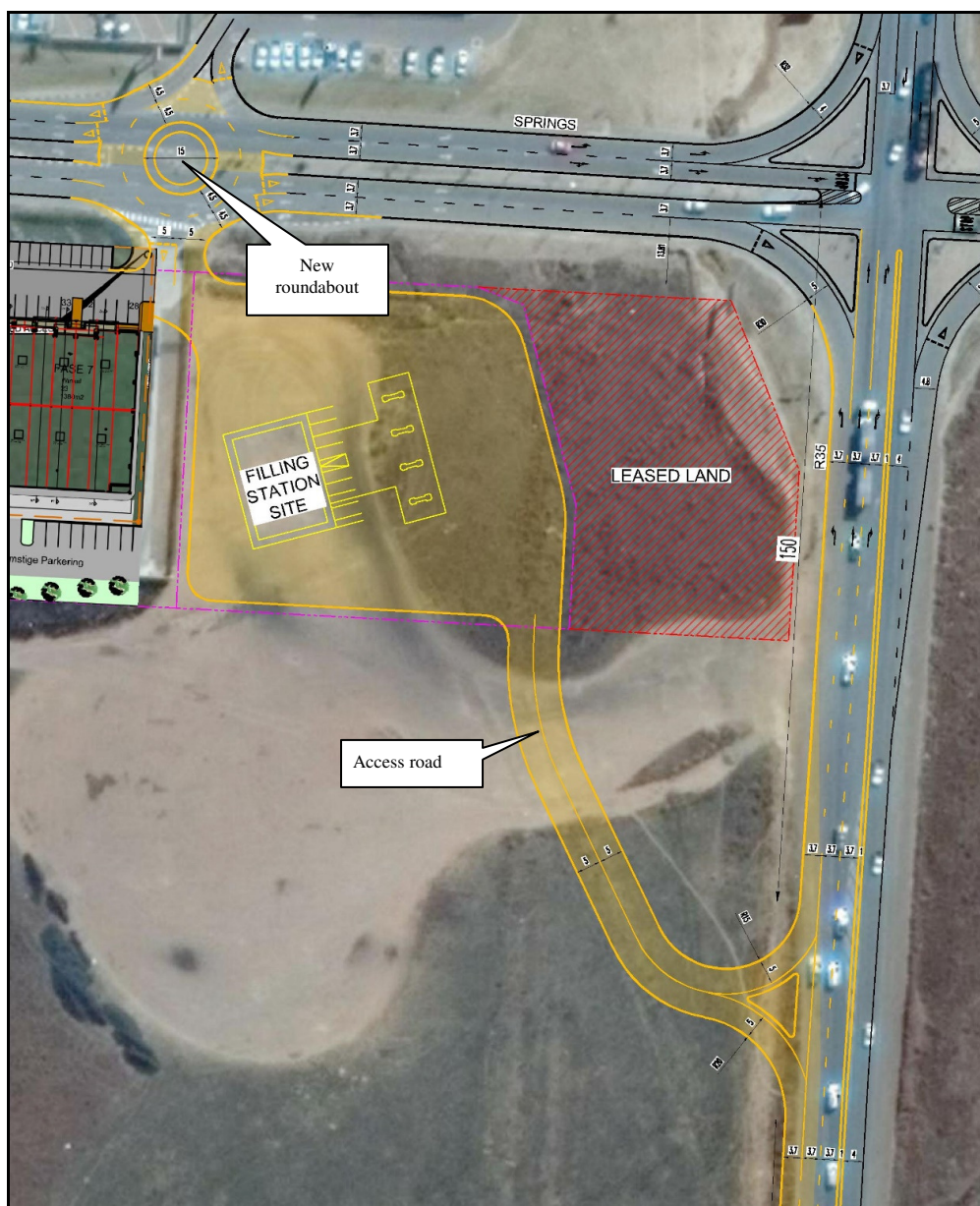
Figure 5.20: Proposed access from Samora Machel Street (R35) and La Roca Boulevard (taken from Roberts, 2017)
