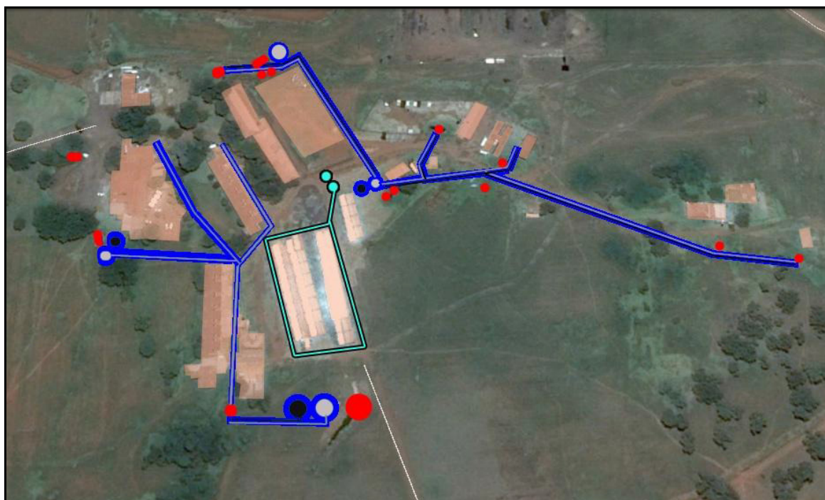
Figure 2.3: Location of septic tanks (indicated by red dots) on site
