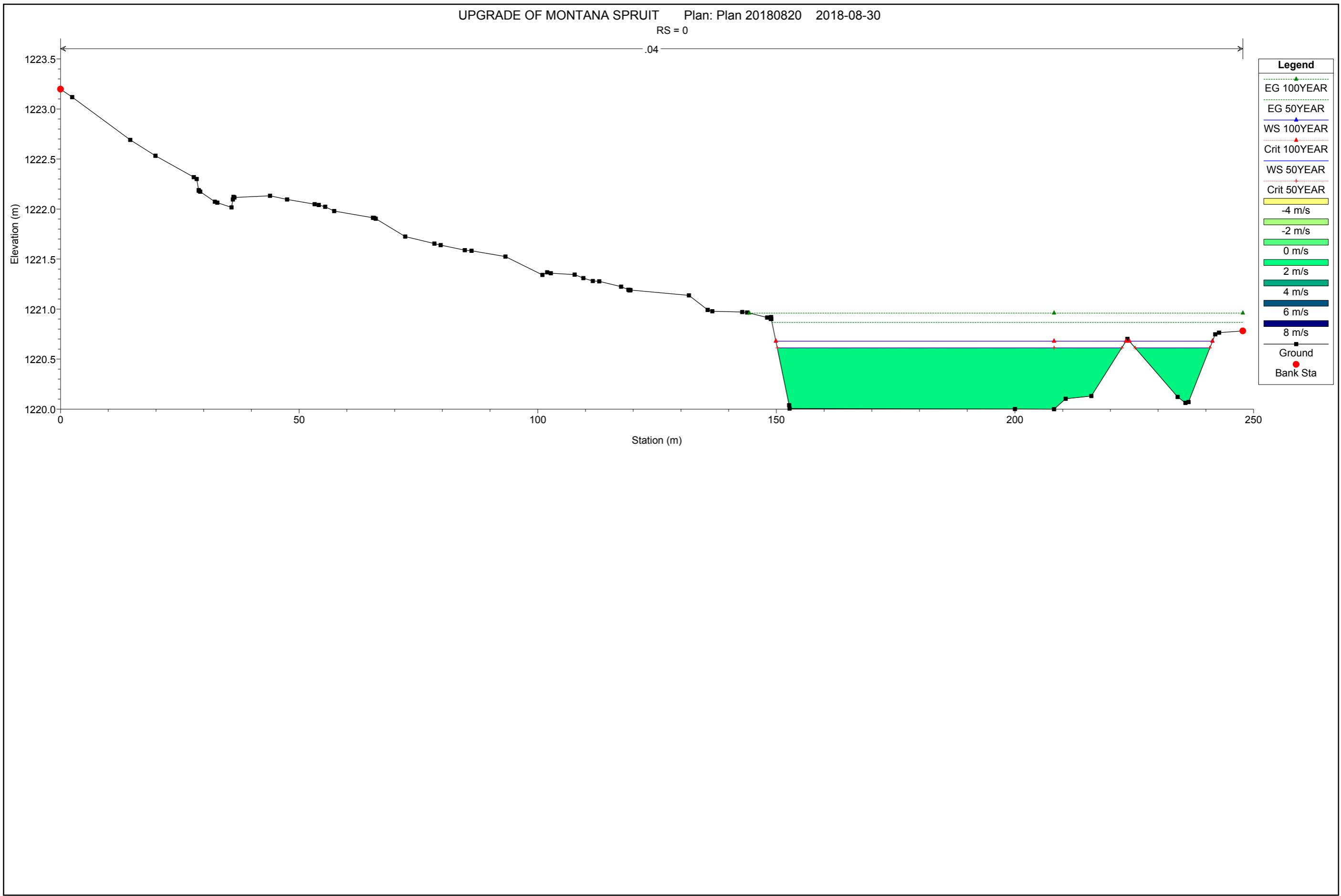
Plan: Plan20180820 V2 08-17 07-12 RS: 622.45 Culv Group: Culvert #1 Profile: 100YEAR
