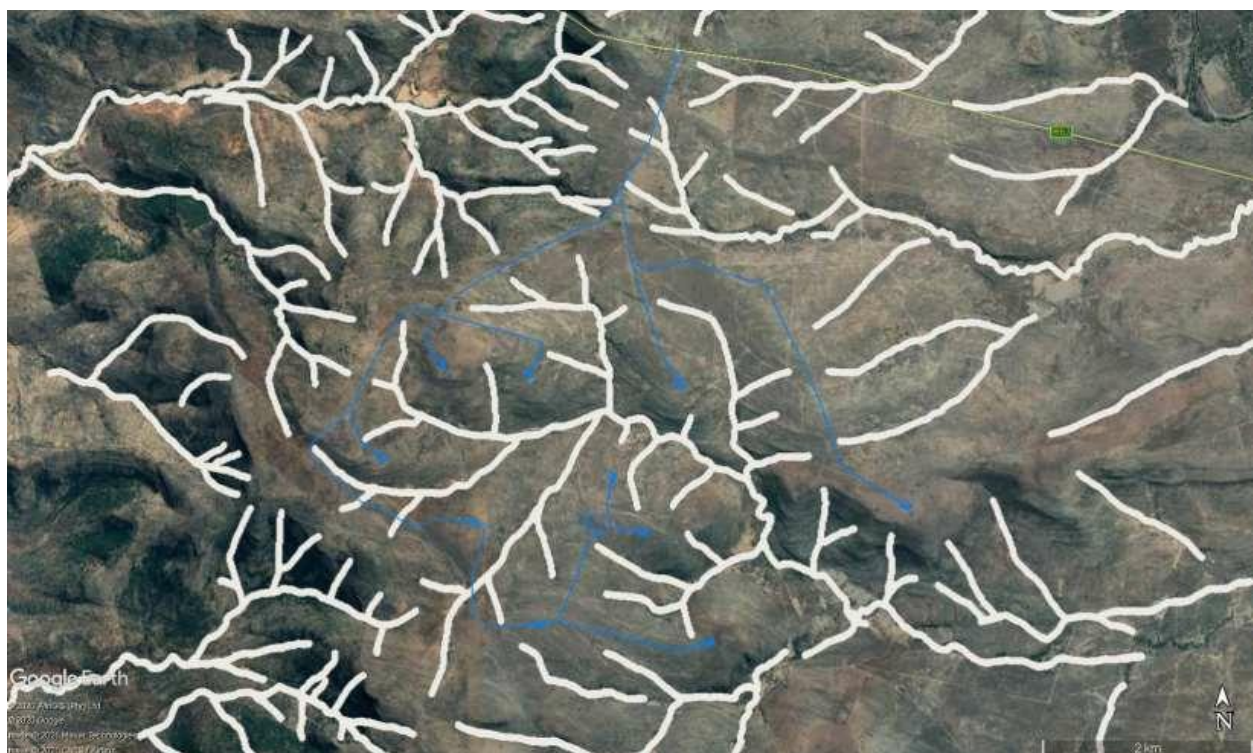
Figure 5: Proposed amended layout (blue lines) when compared to the observed watercourses with 32 m buffer (Source: Colloty, 2021)
