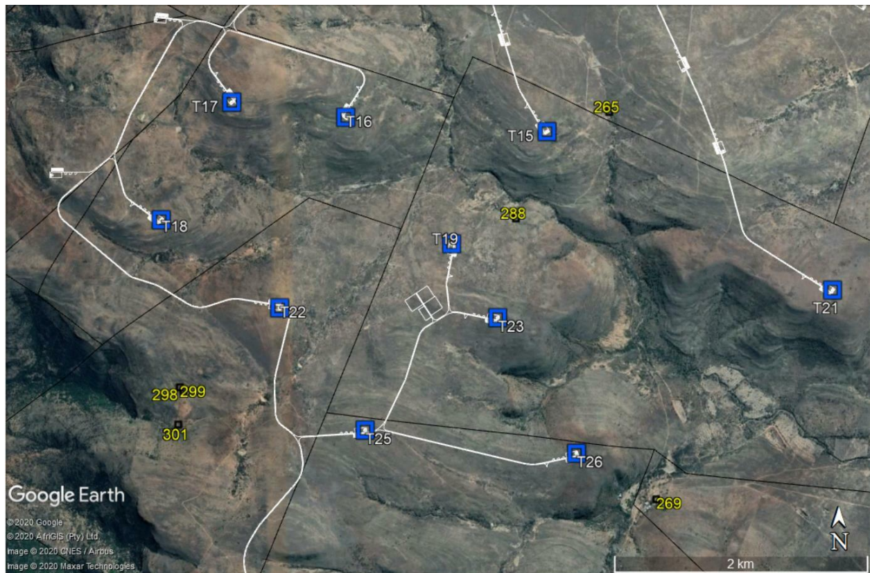
Figure 7: Aerial view of the proposed Highlands Central WEF showing turbine locations (blue numbered squares), facility layout (white lines (note that the adjoining Highlands North WEF is also included but its turbines are not shown)), and palaeontological resources (numbered black squares) (ASHA Consulting (Pty) Ltd).
