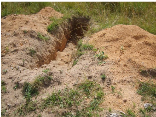
Photo#3: Geo-Tech test pit
