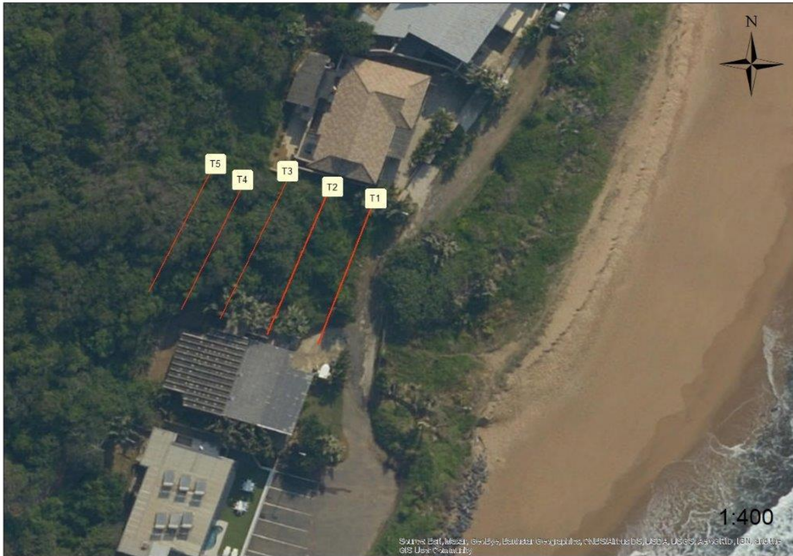
Figure 7. Map image detailing the transect layout across the subject site representative of elevation and distance from the ocean.
