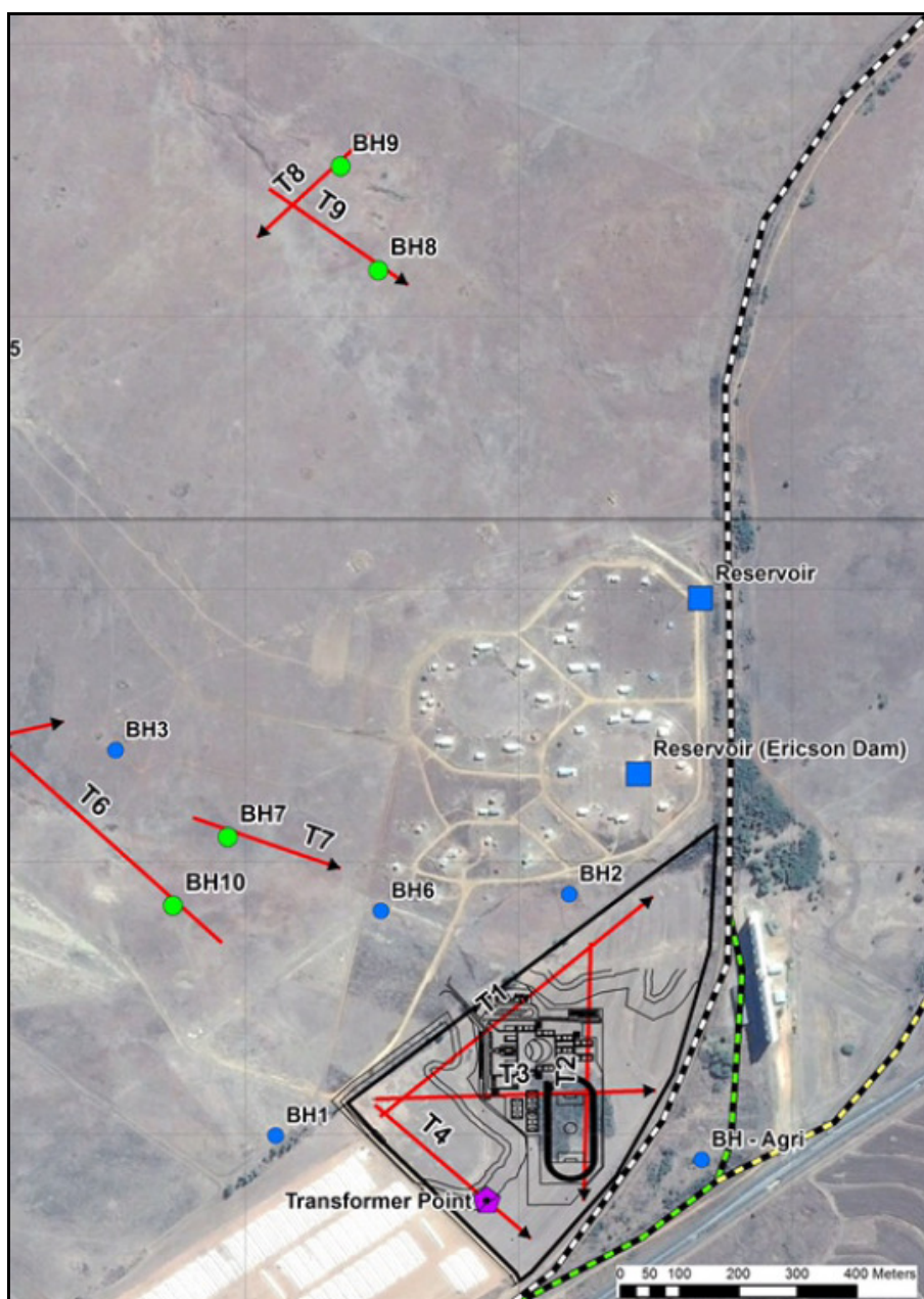
Figure 5.18: Location of the newly drilled boreholes (taken from Du Preez, 2017)
