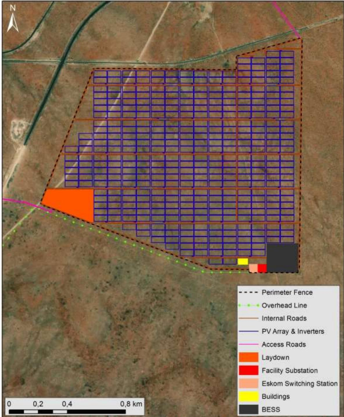
As can be seen above, the proposed BESS is situated in the South East of the approved footprint, adjacent to the on-site substation. The full-sized layout plans are appended to the Amendment Assessment Report and application for amendment form.
