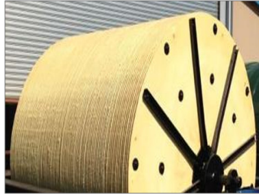
Figure 5-3 A complete rotor unit – visible are blades, spiders, through rods, shaft and bearing
