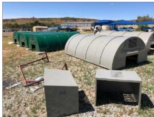
Figure 5-4 Rotor and gearbox covers in various colours
