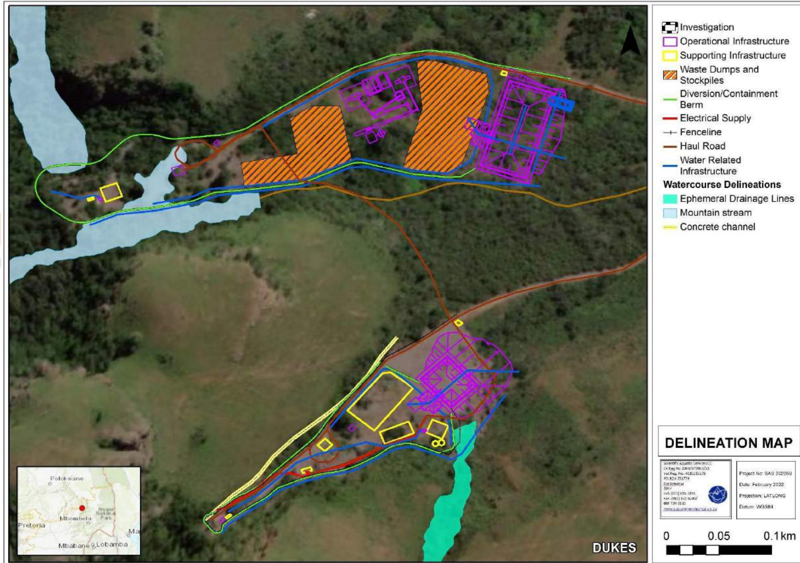
Figure 82: Identified freshwater ecosystems within the Dukes UG area and associated investigation area, in relation to the surrounding landscape
