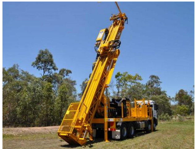
Figure 2: Typical core drilling rig
