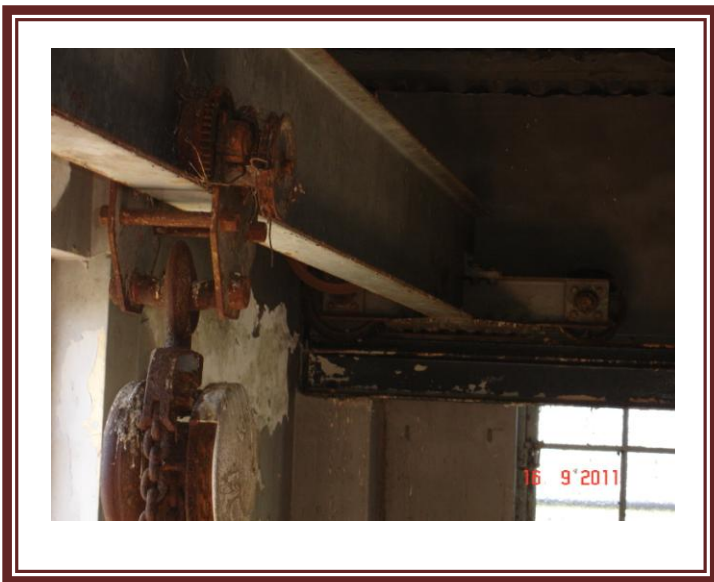
Fig.22. Hoist runner along gantry and gantry gear and pulleys left.
