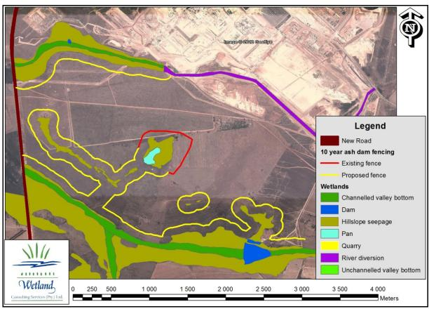
Figure 2. Map showing the updated wetland delineation as well as the required 100m buffer zone along which additional fencing should be installed. The section of fence to be removed is also shown.
