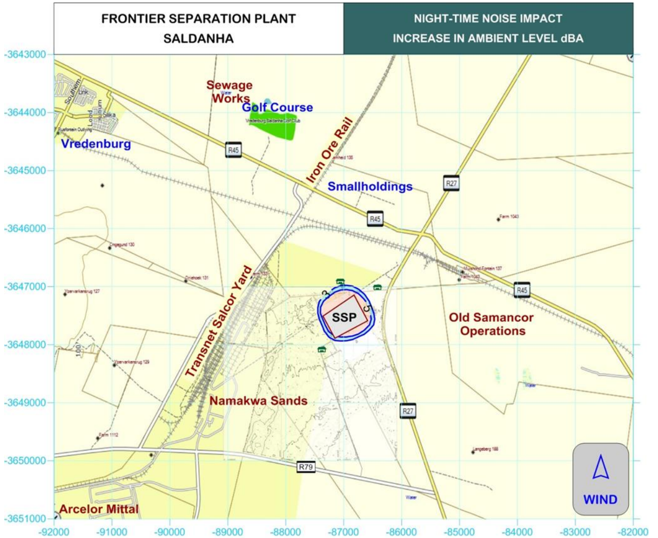
Figure 7-10 Noise contour map (indicating impact insignificant outside the 3 dB contour and inside the 5 dB contour)
