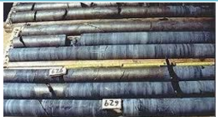
Rock core recovered for analysis
