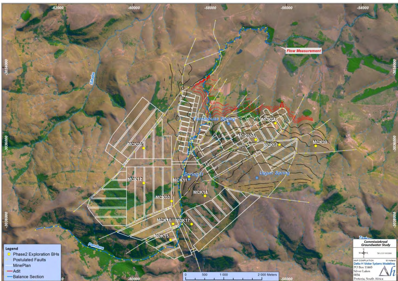
Figure 7.4: Pandana River balance section and flow measurement location.
