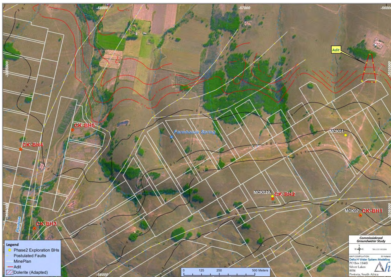
Figure 3.3: Positions of newly drilled boreholes in relation to proposed mine workings.
