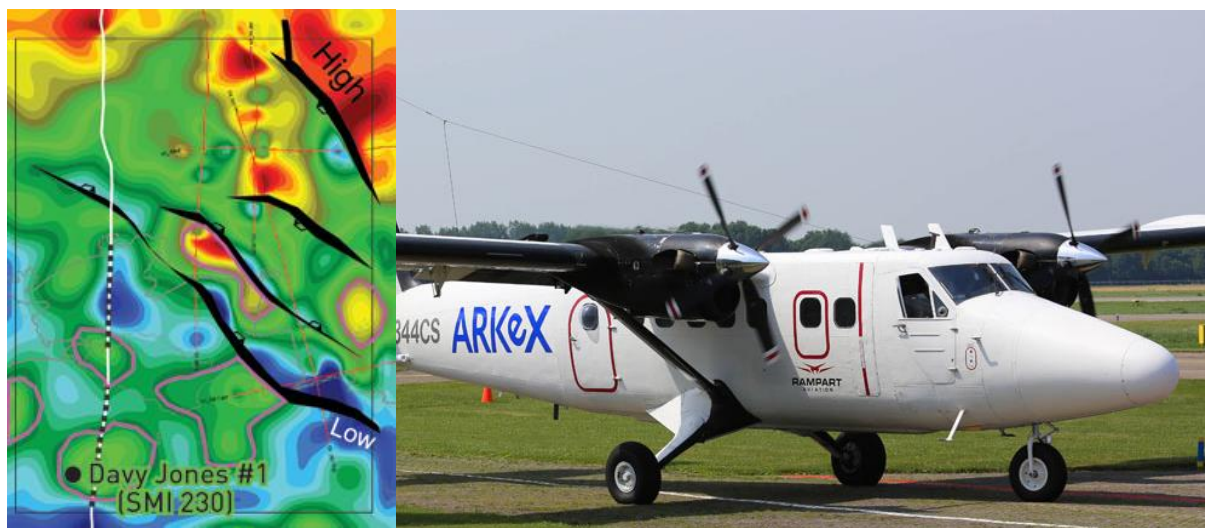
FIGURE 4-2: TYPICAL FTG EQUIPMENT AND RESULTS
