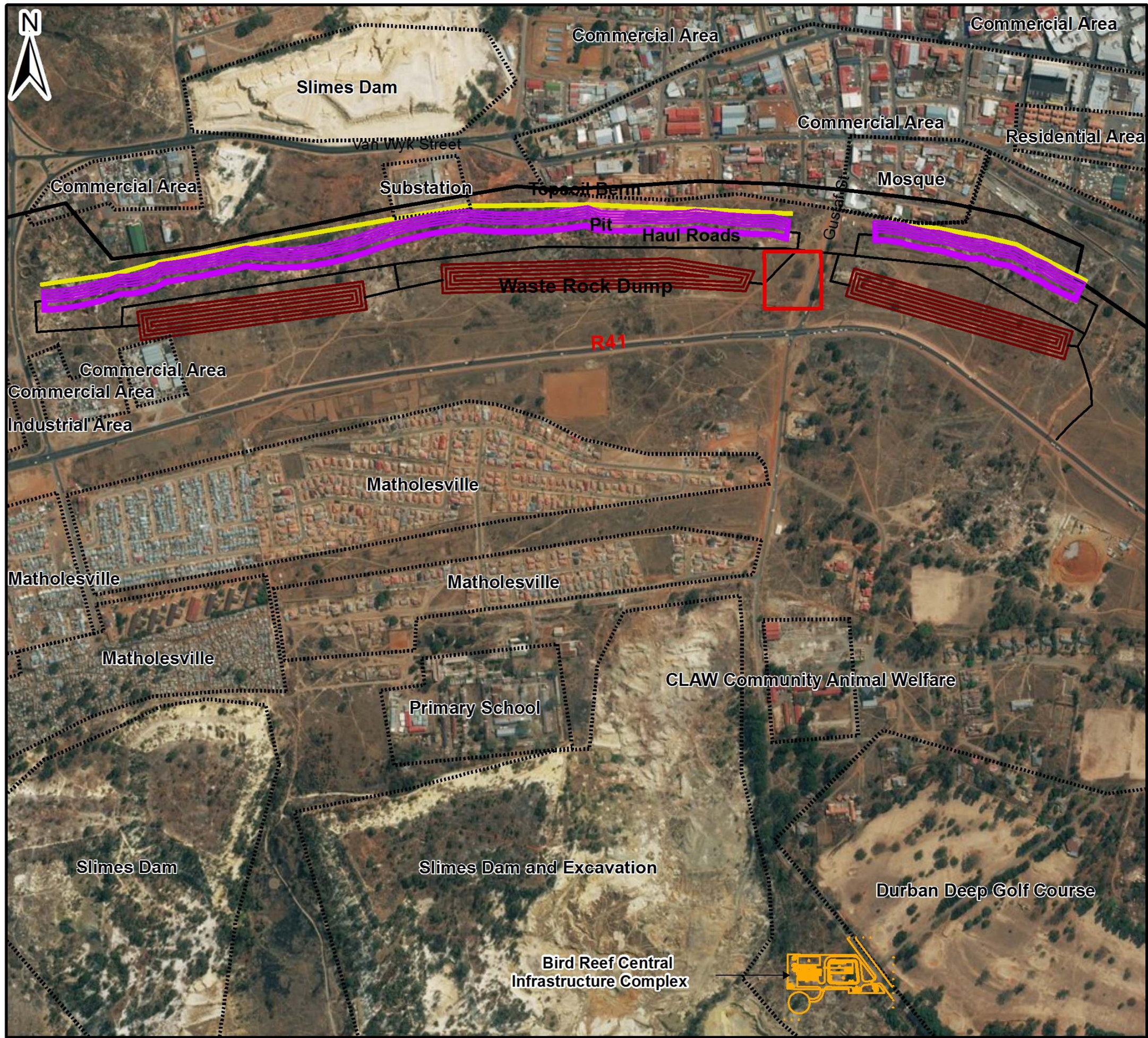
Figure 4 Conceptual Design Layout of the Proposed Roodepoort Main Reef Pit and the Bird Reef Central Infrastructure Complex
