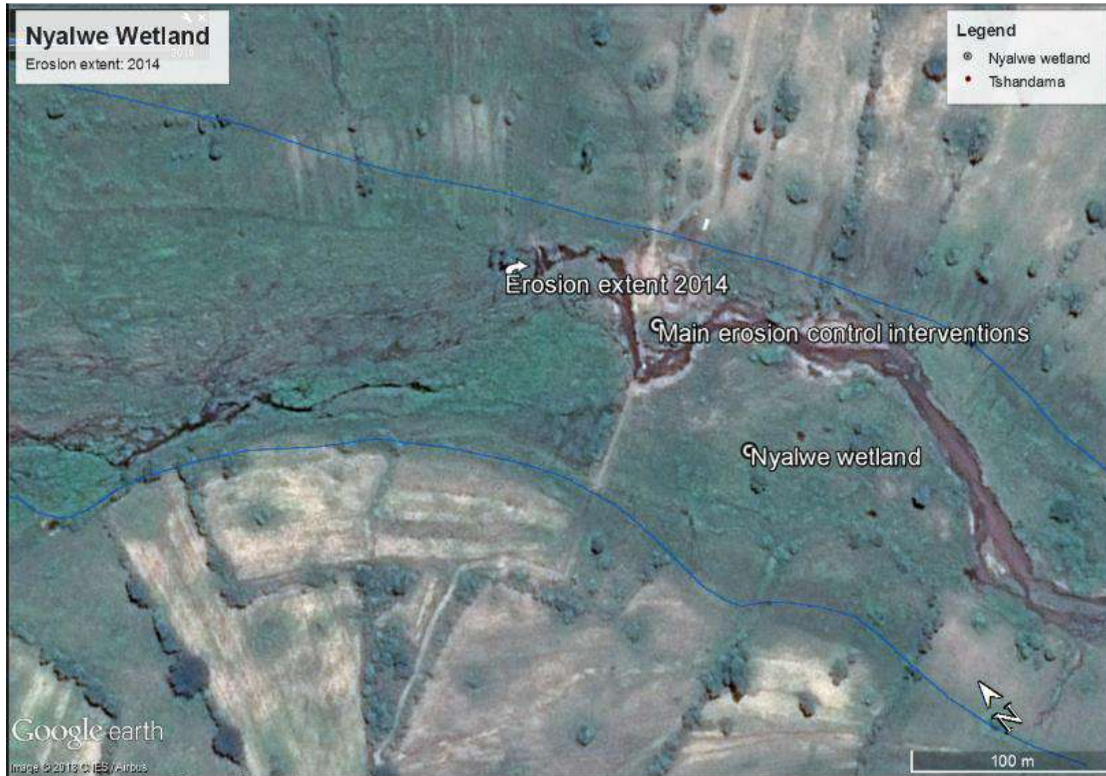
Figure 5: The extent of gully erosion in 2014. Rehabilitation measures were upgraded during this period.
