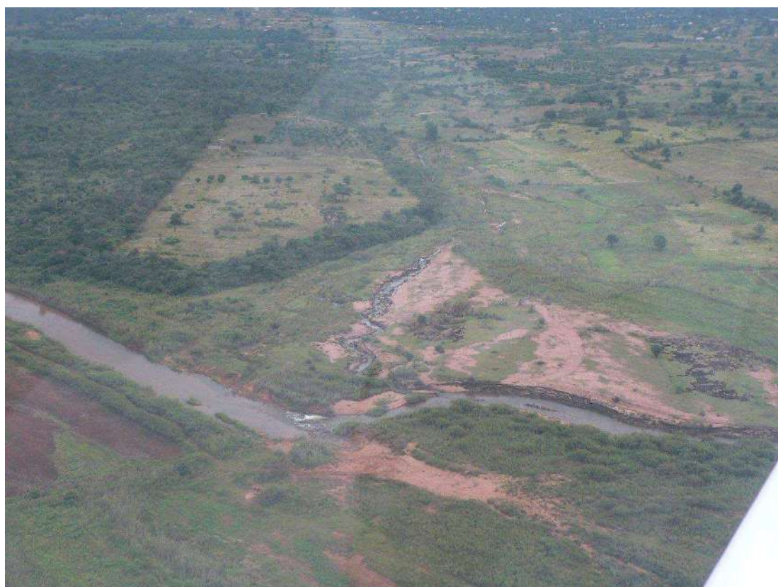
Figure 7 - Headcut and Donga erosion, as well as excessive sedimentation in the Mutale
