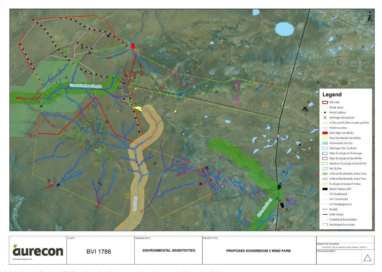
Figure 1: Authorised layout for Kokerboom 2 Wind Farm and associated infrastructure superimposed over mapped environmental sensitivities
