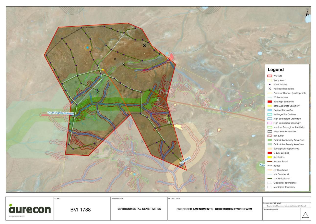
Figure 2: Proposed optimised (amended) layout for Kokerboom 2 Wind Farm and associated infrastructure superimposed over mapped environmental sensitivities
