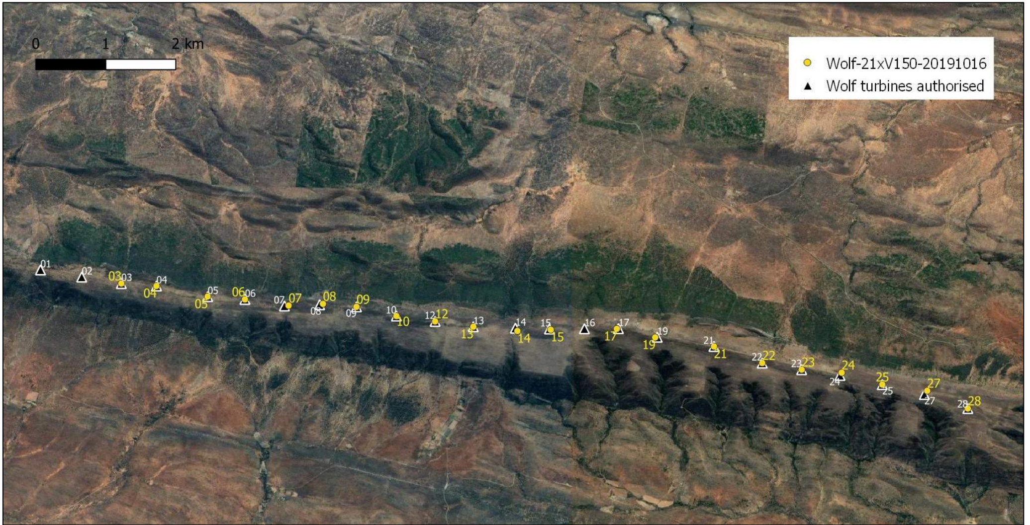
Figure 3-3. Comparative turbine layout (original – white; new – yellow).
