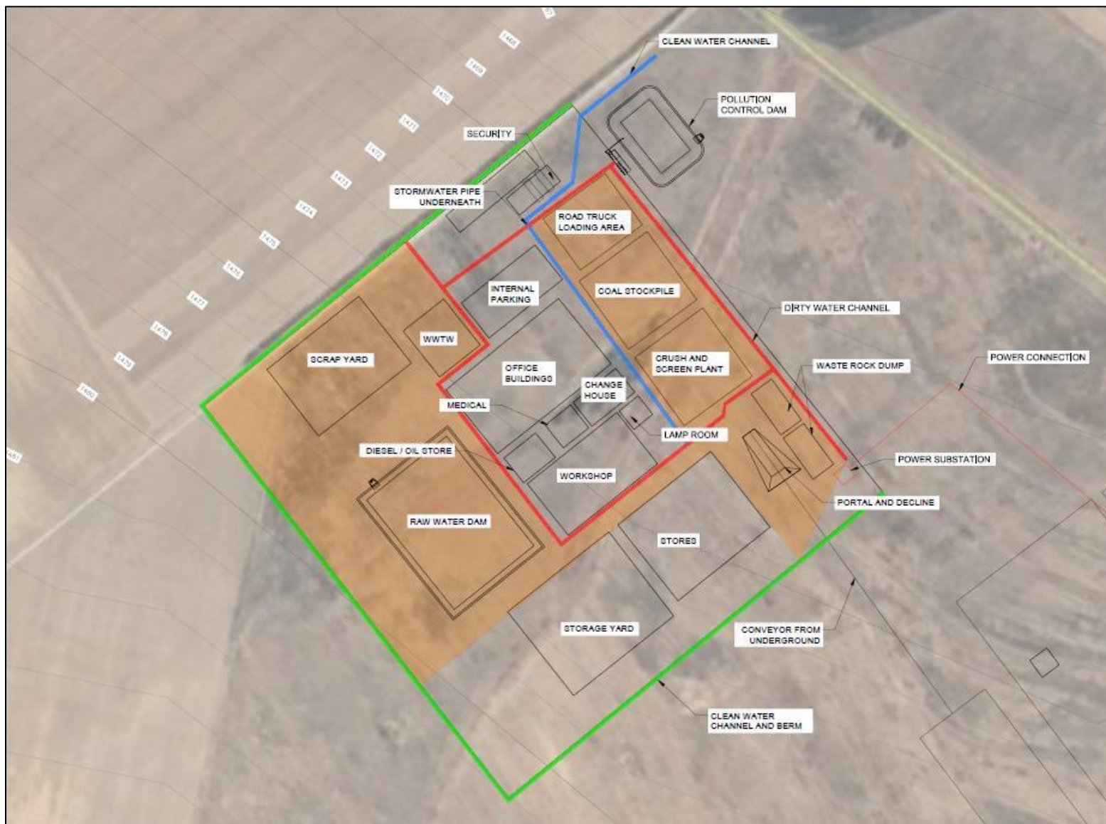
Figure 7-3: Final formal designed Engineering Layout (Part of Phase 3 Designs for WUL process)
