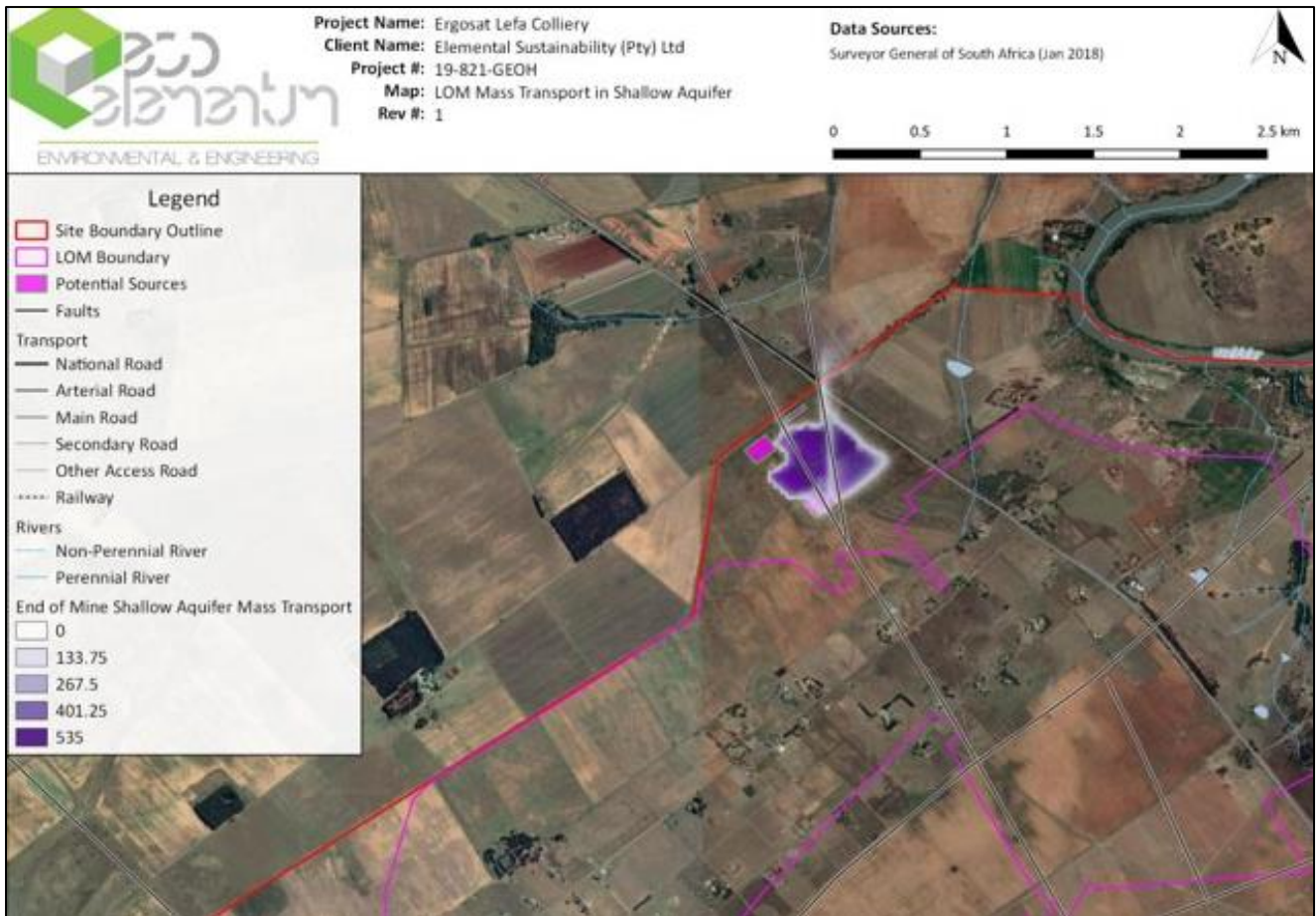
Figure 10-26: The simulated mass transport at the end of the operational phase in the shallow aquifer at Lefa Colliery
