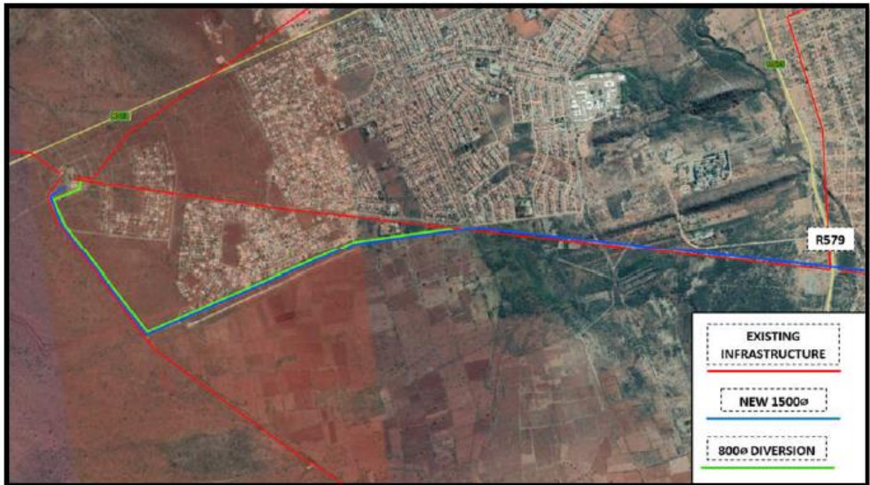
Figure 7: Diversion along Lebowakgomo S.
