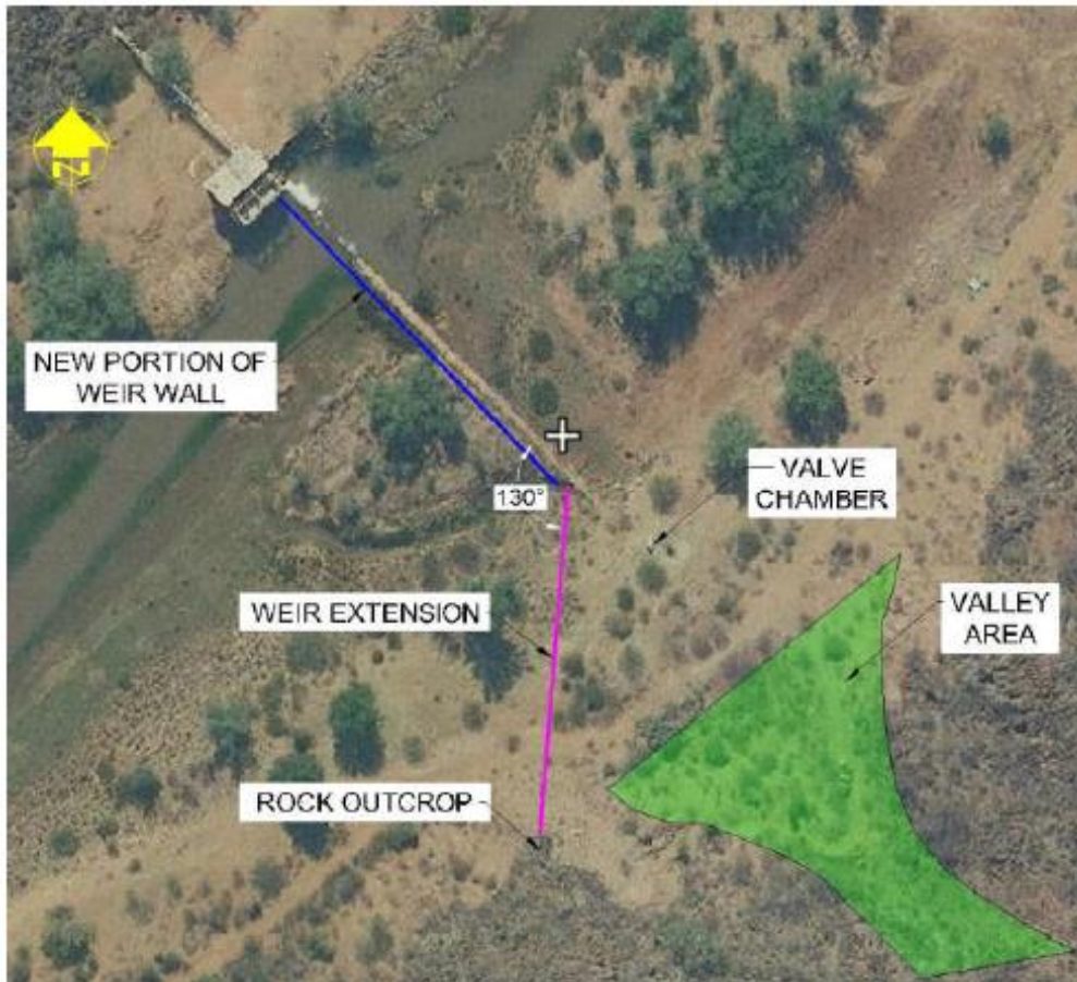
Figure 10: Upgrading of weir design
