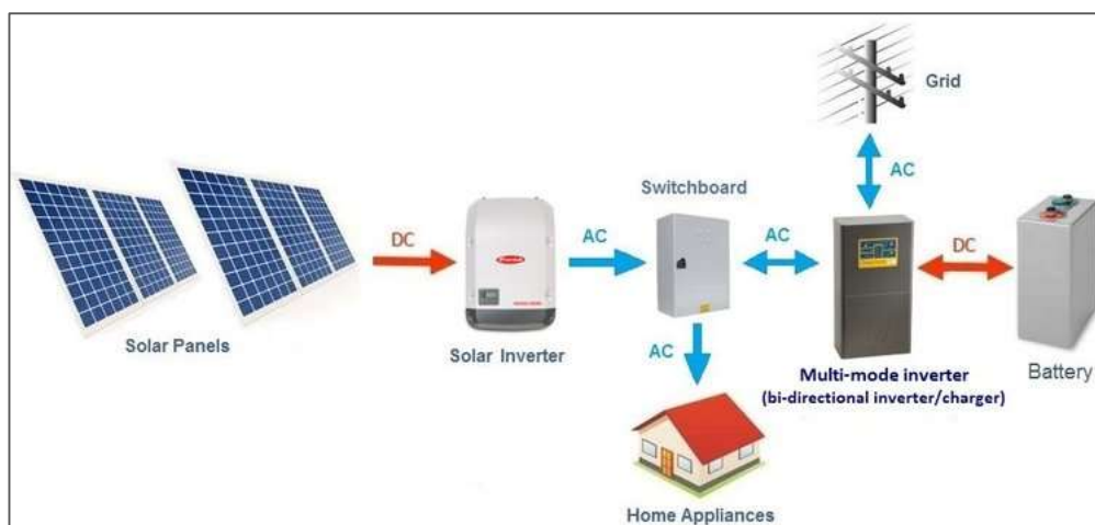
Figure 5-3: A process diagram illustrating the usage of a BESS in the electric grid.
