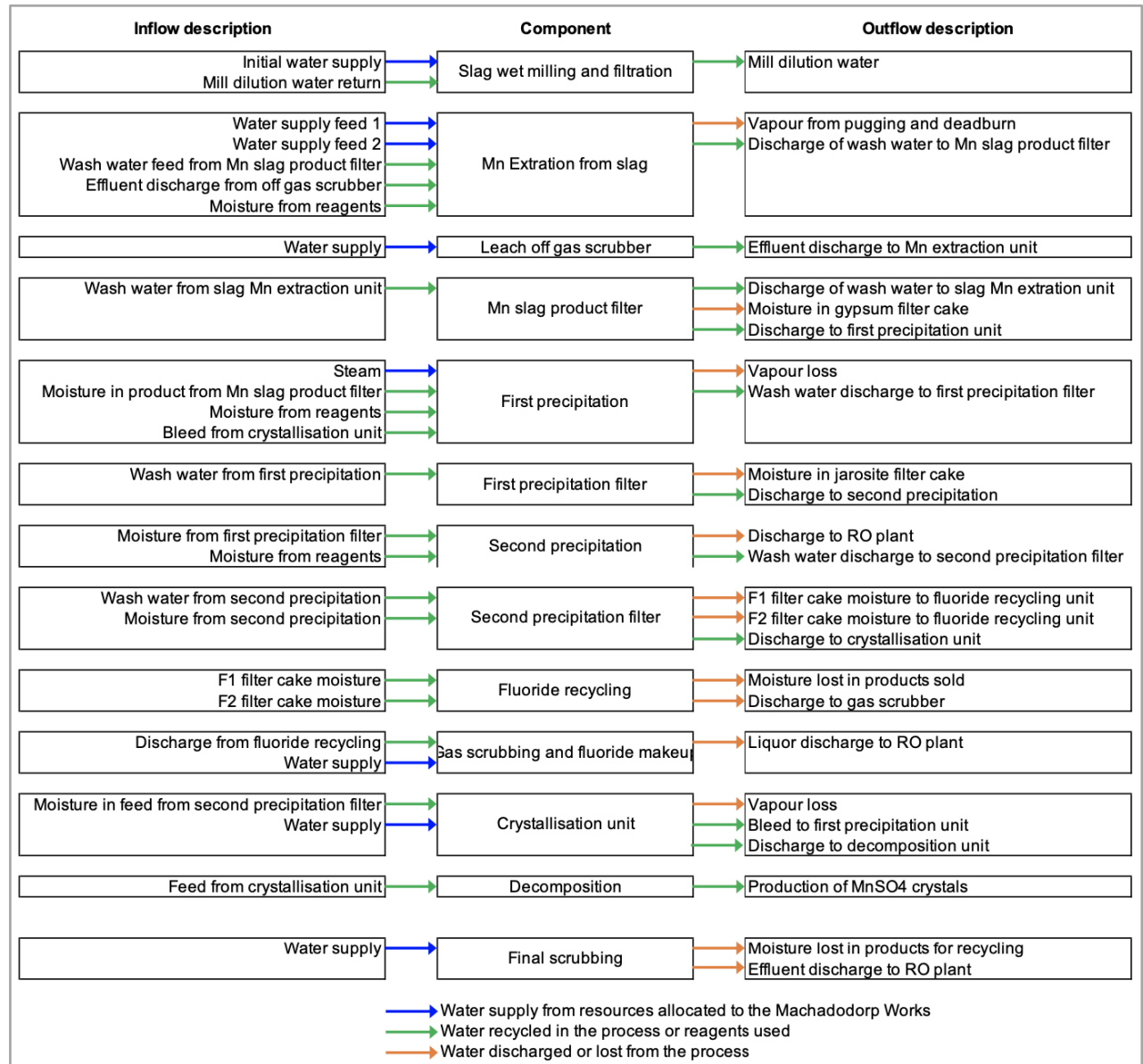
Figure 6 Conceptual water balance for the MnSO 4 Recovery Project
