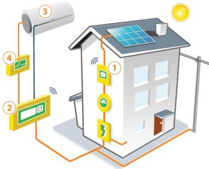
Figure 31: Household Geyser Solar System
