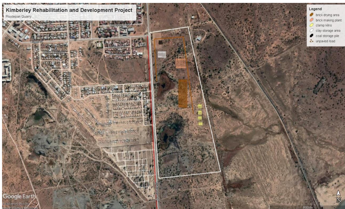
Figure 9: Assumed site layout of activities at Roodepan Quarry and Clay Brick facility
