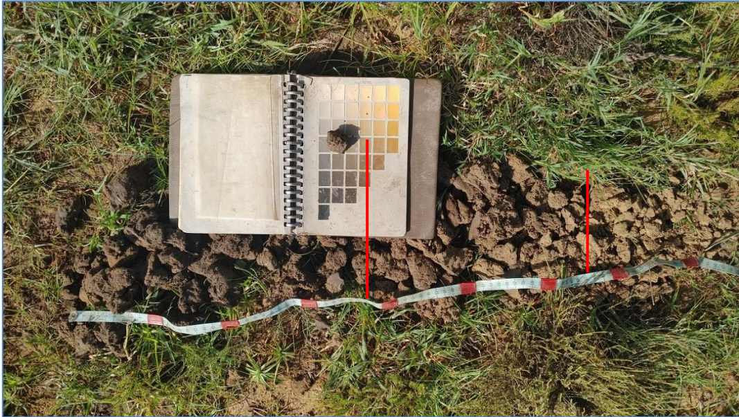
Figure 14: Image illustrating from left to right, the Melanic A horizon, followed by the G 1 and G2 horizons of the wetland soils
