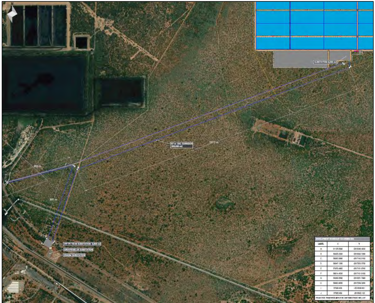
Figure 1-4: The position of the proposed Lephale Solar PV Facility relative to the connection point at the Grootegeluk Substation as well as array relative to the proposed high voltage powerlines connecting the Solar Power Plant to the Grootegeluk substation (provided by client).
