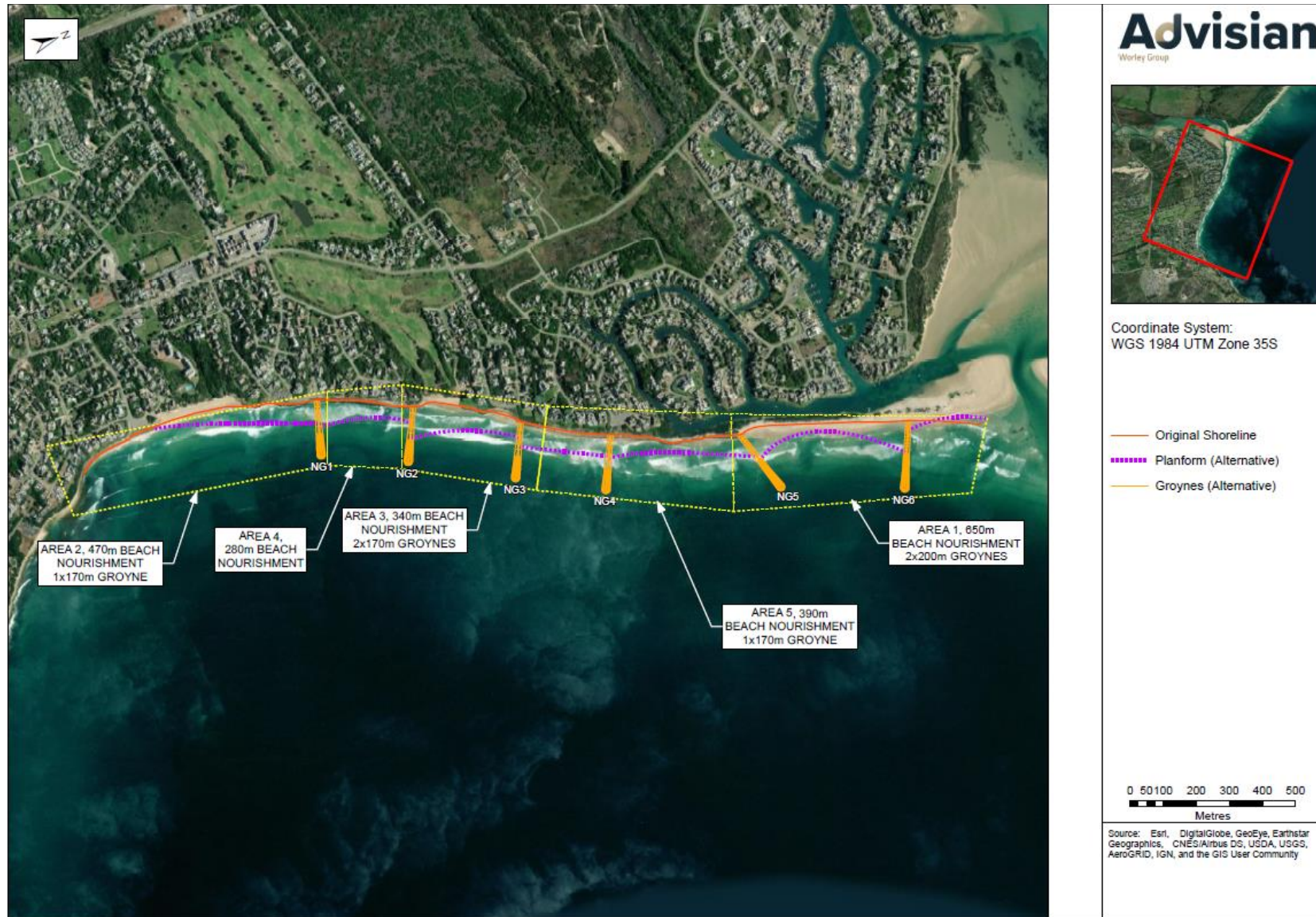
Figure 4.3: Proposed layout for the stub groyne
