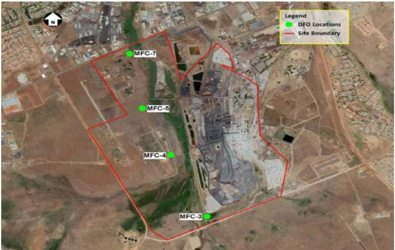
Figure 12: Location of dust fallout monitoring points
