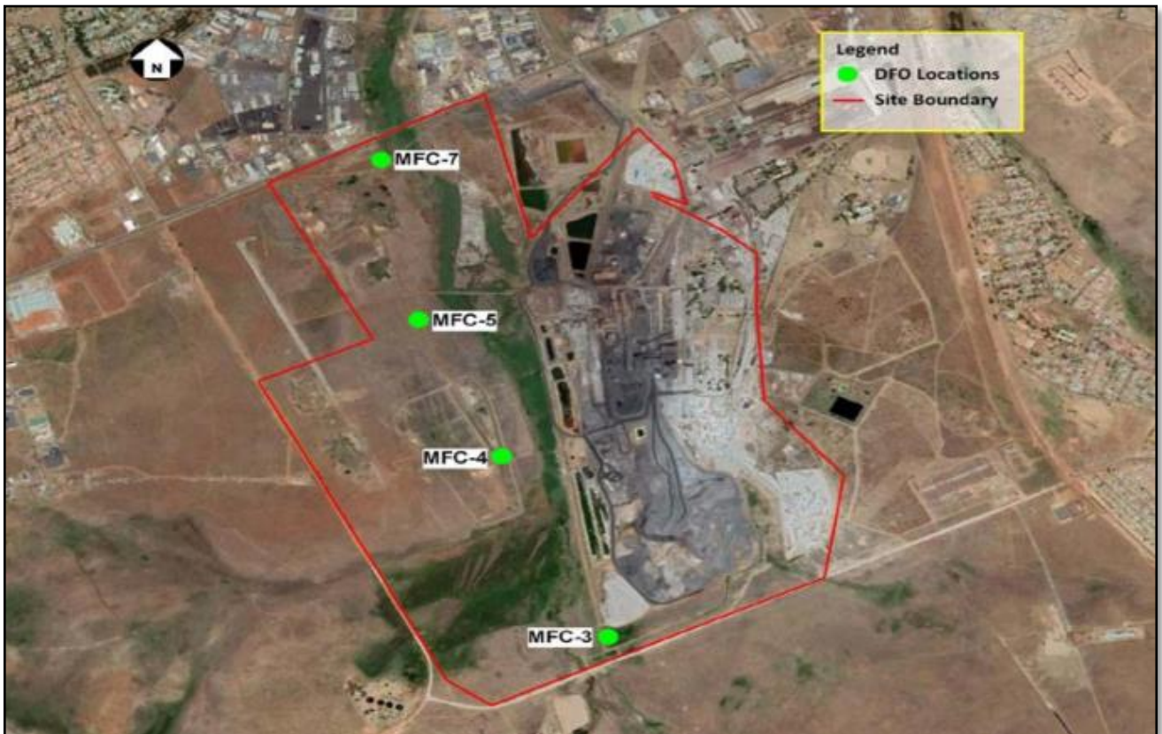
Figure 16: Location of dust fallout monitoring points
