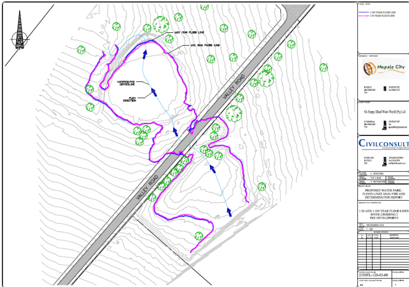
Figure 4-8: Valley Road Watercrossing and post development floodlines
