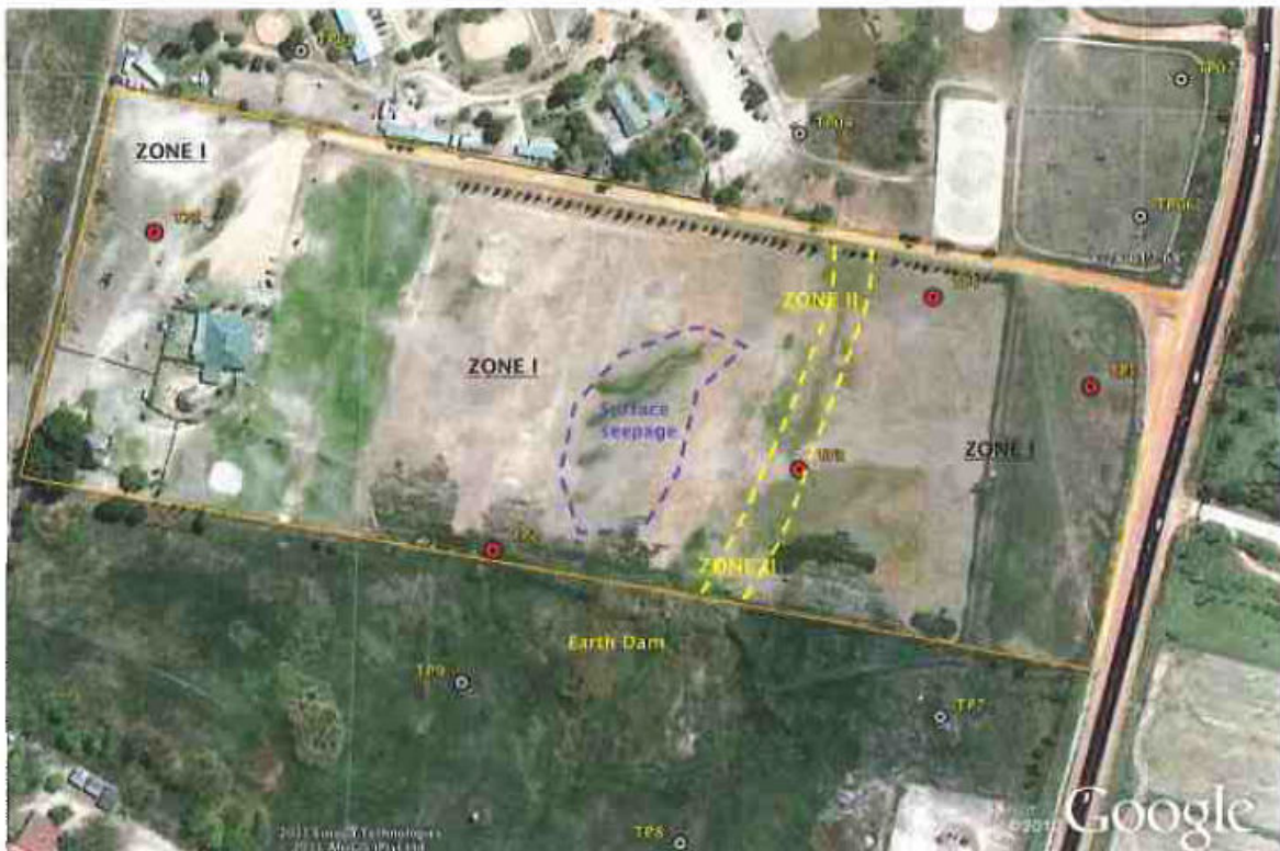
Figure 9-10: Test Pit Locations and Geotechnical Zoning
