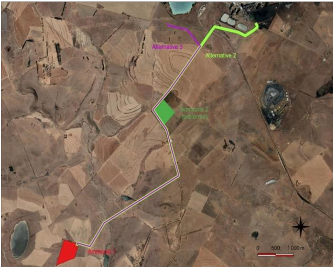
Figure 7: Pipeline alternatives for Ammonia 1.
